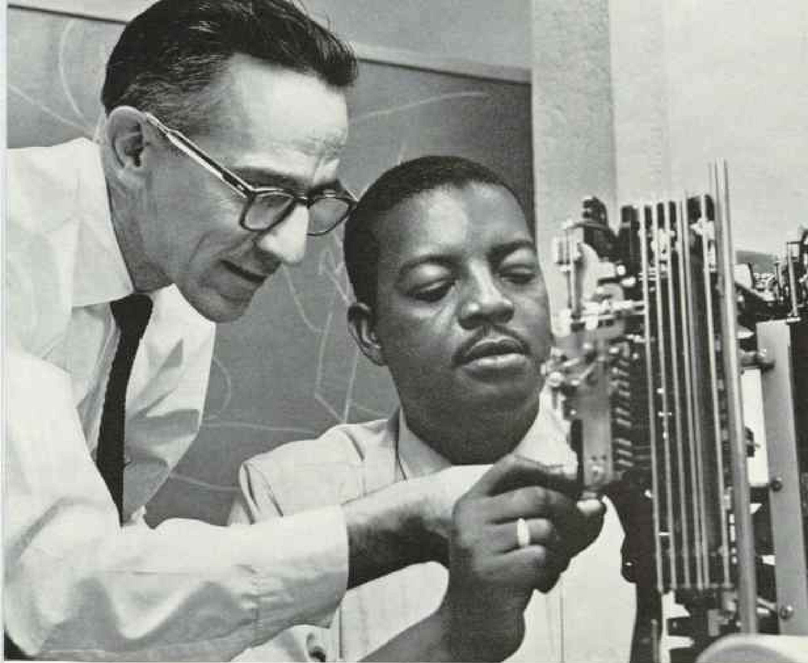
Bell System instructor George Templeton, left, discusses maintenance problems of a teletypewriter printing unit with Henry A. Louz of Surinam, who has come to this country to receive advanced communications training.
