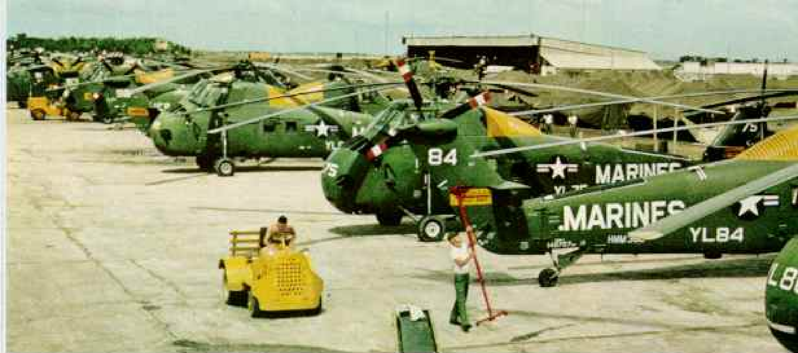
Fighting against time, Marine crews repair helicopters at Khanh Hung on a rare morning when the machines are grounded. For safe operation, every hour of flight requires about 12 hours of maintenance.
