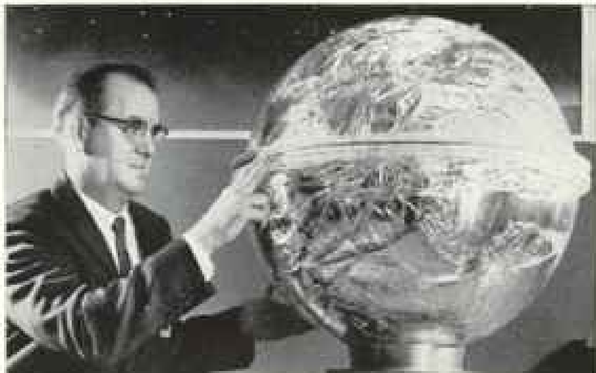
Transparent display sphere encases a satellite made of thin aluminum-coated plastic. Fired into orbit, the satellite pops from a container and expands to a diameter of 100 feet.
