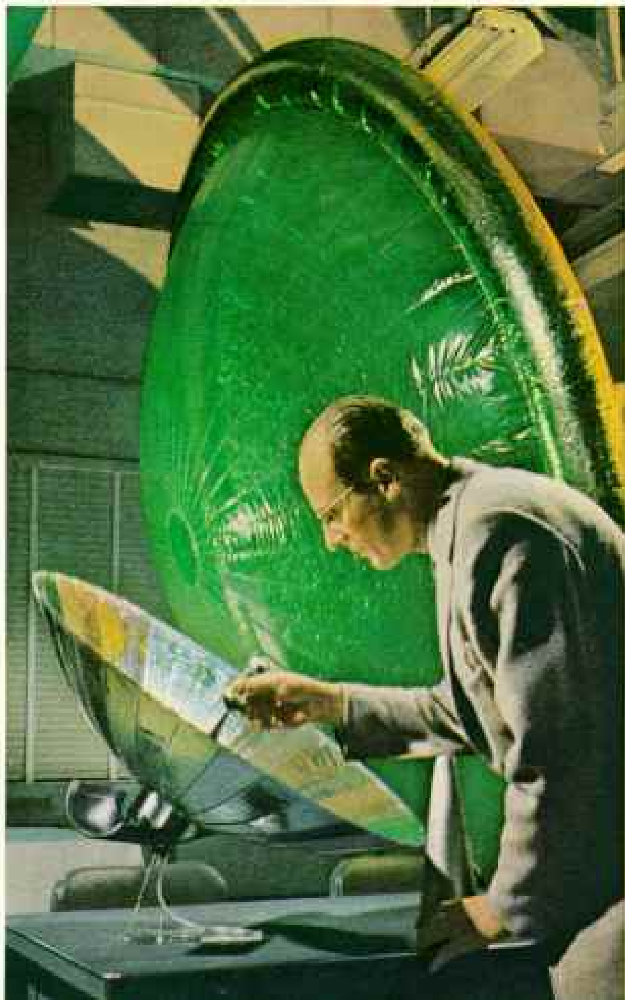
Umbrellalike reflectors of paper-thin plastic may be used as space antennas or solar heating units. Scientist Walter J. O'Sullivan of Langley, who conceived the idea of plastic satellites, examines a model. The reflector would gather sunlight and convert its heat to electricity for broadcasts. Larger model in background is an antenna.
