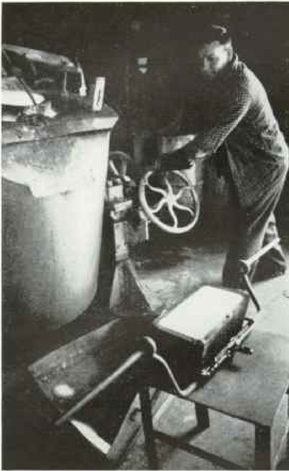
Pouring gold, a worker in Fairbanks rights the kettlelike crucible after filling a mold with metal heated to 2,000° F.
