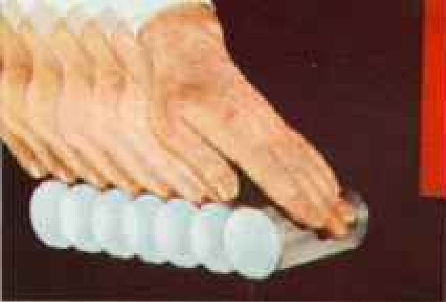
OLD WAY WITH KING PINS —A pin rolls freely in only two directions, restricts easy, 4-way front-wheel motion on conventional cars.
