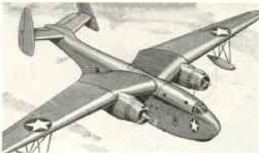
3 Fast Freight reaches fighting fronts quickly in this two-engine Navy transport. Big sister of plane No. 2 above, she has similar silhouette but weighs four tons more, lacks gun-turrets. Could you spot this plane? See answer at lower left.
