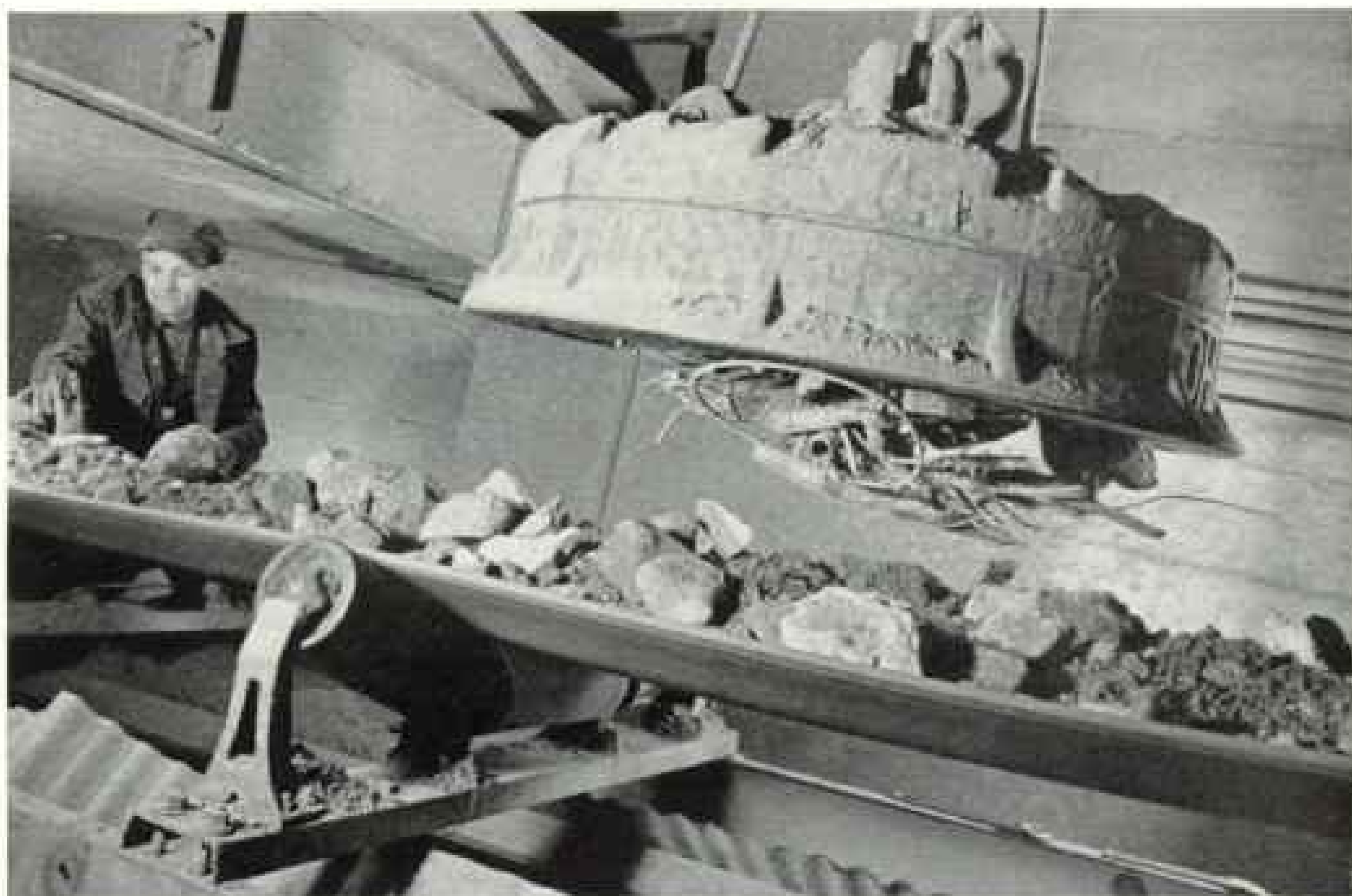
Powerful Electromagnets Pick "Tramp" Iron from Copper Ore on a Conveyor Belt Rusty old spikes, pieces of wire, and bits of broken tools are extracted automatically from the ore stream.
