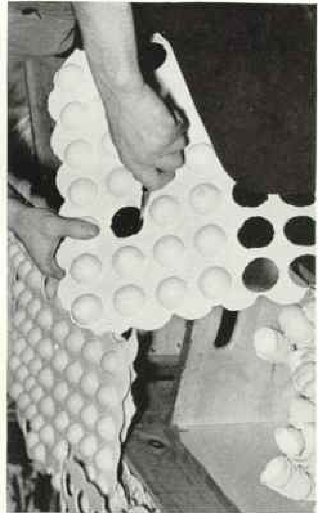
SOLID CORES ARE UNLOADED AFTER VULCANIZING Sometimes hollow centers are filled with liquid.
