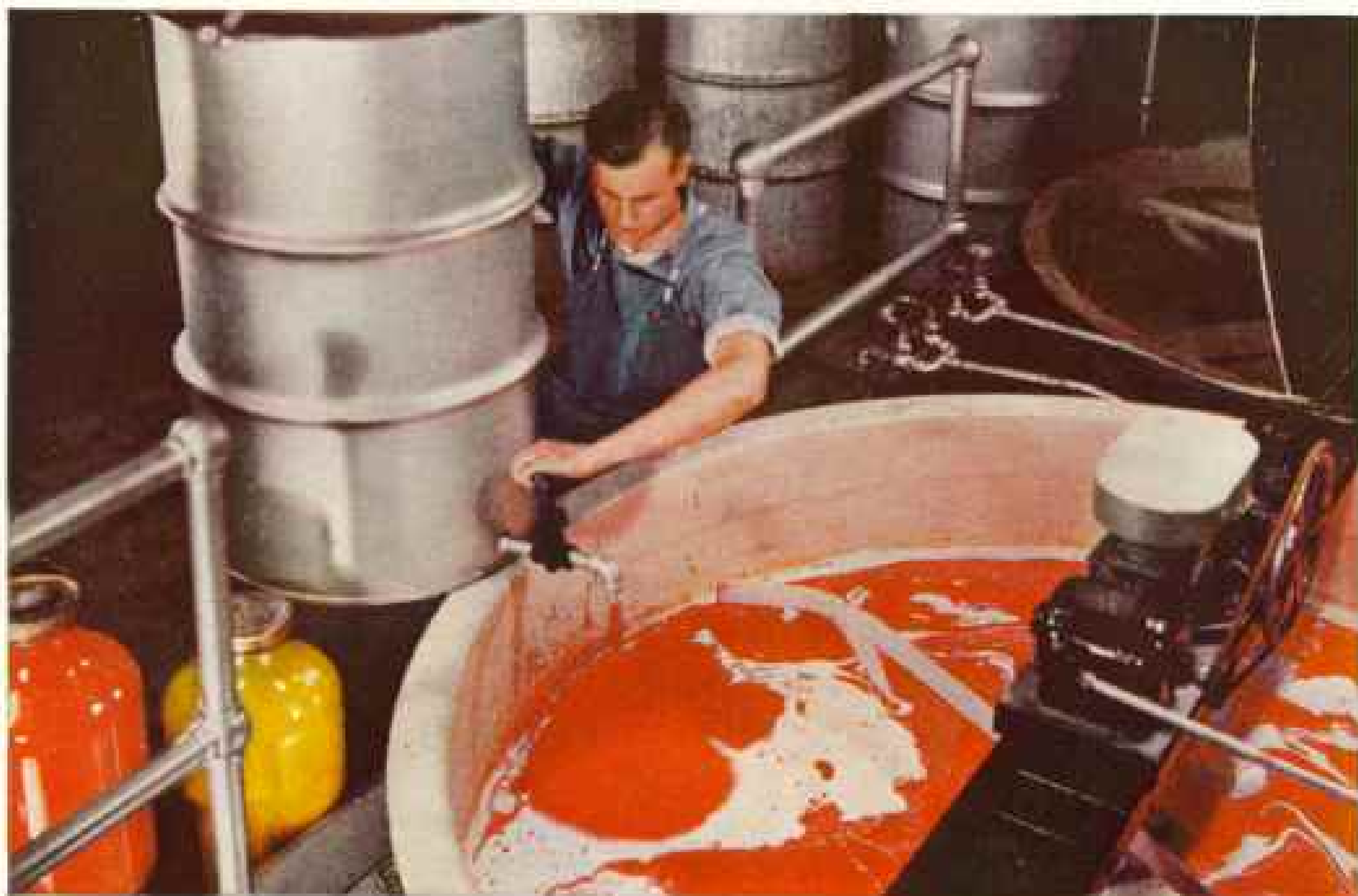
RUNNING A COLOR BATH FOR A TANK OF EMBRYO TOY BALLOONS
