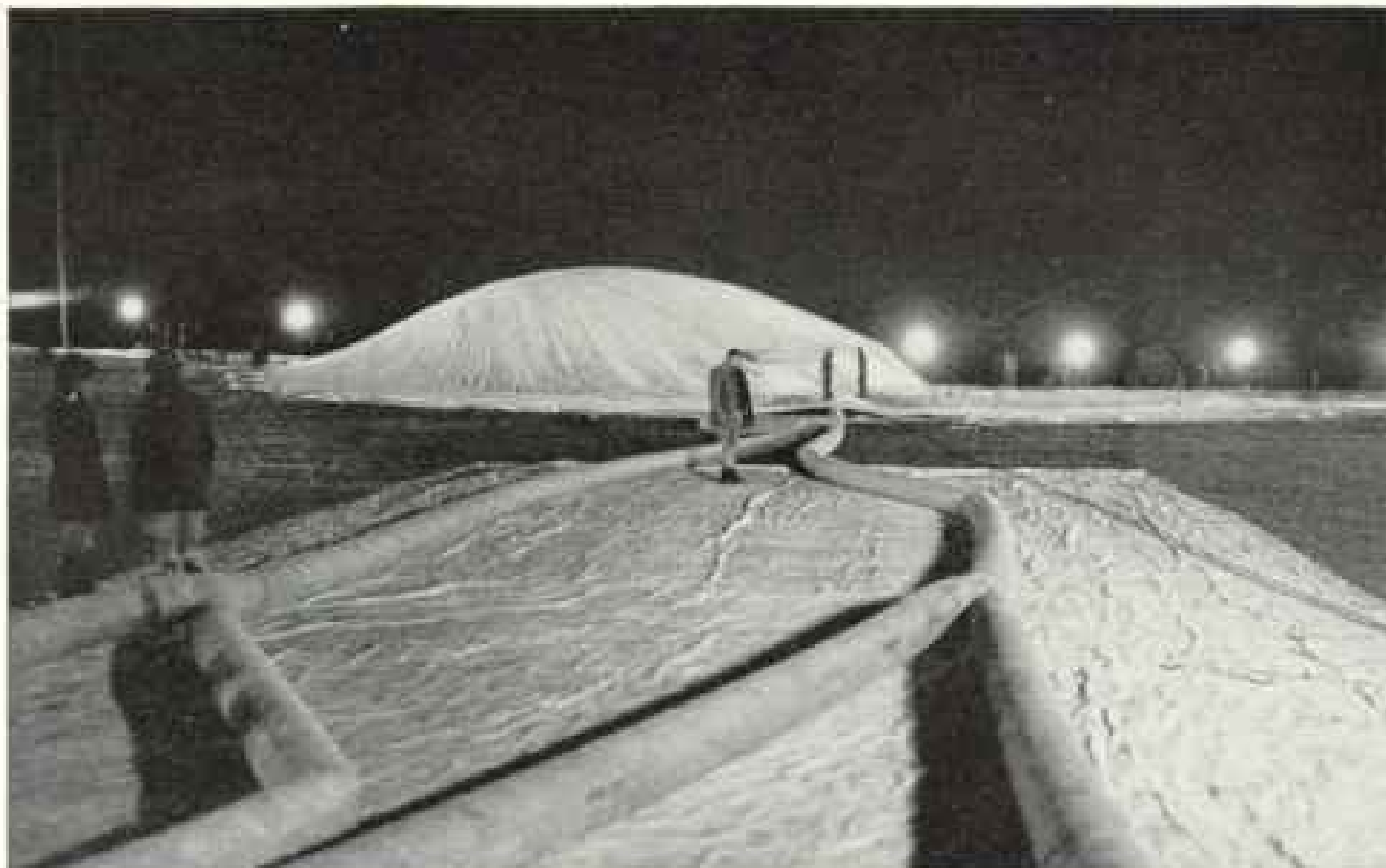
SERPENTLIKE HOSE CARRIED HELIUM TO THE BAG
