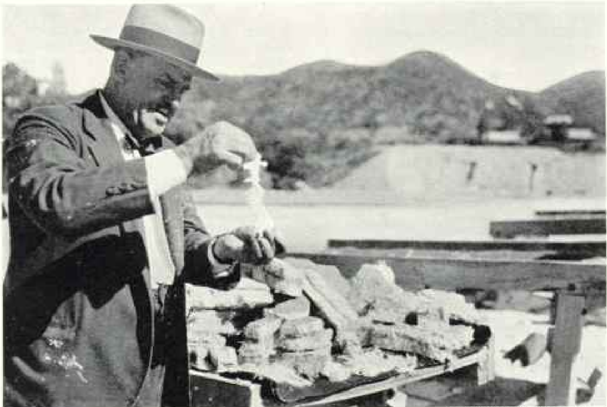
ASBESTOS CHUNKS, FRESH FROM THE MINE, ARE SAMPLED FOR THE FIBER'S SPINNING LENGTH
