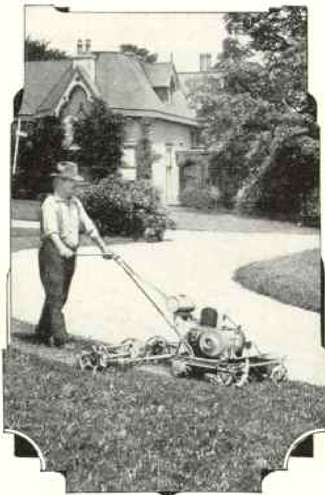
Above: Coldwell "L-Twin" Motor Mower and Roller. Mows and rolls simultaneously 4 to 6 acres a day. Gang units increase its capacity to 10 acres a day on one gallon of gasoline. Equipped with two cylinder motors.
