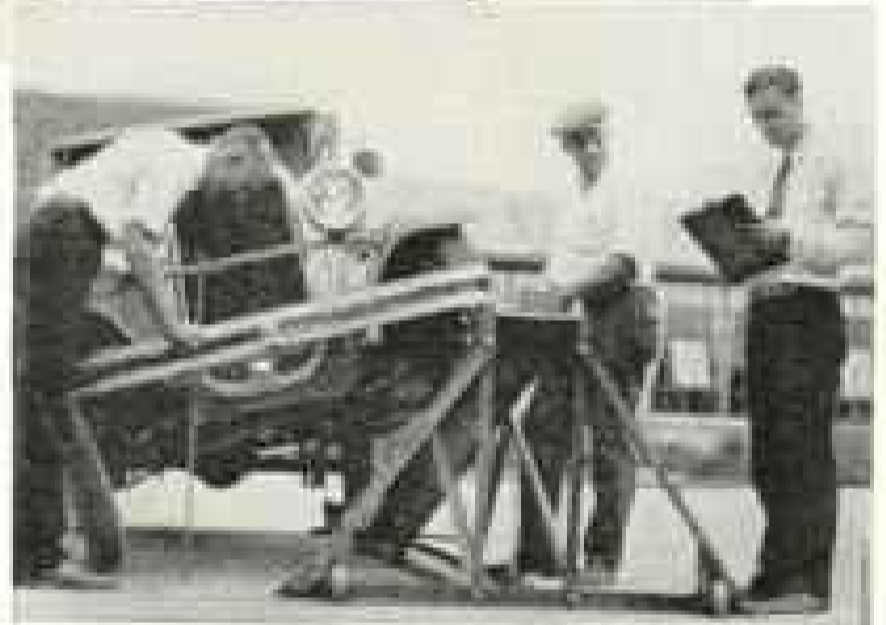
Twisting a car out of shape to determine how stresses and strains affect all parts of it.
