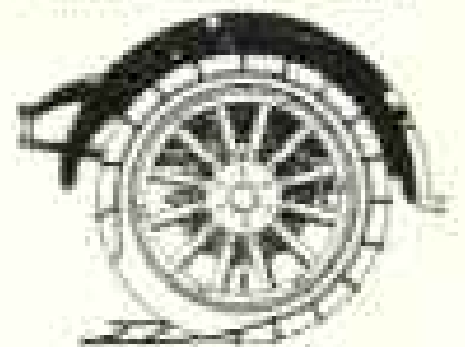
Shift car forward just enough to run over slack ends.
