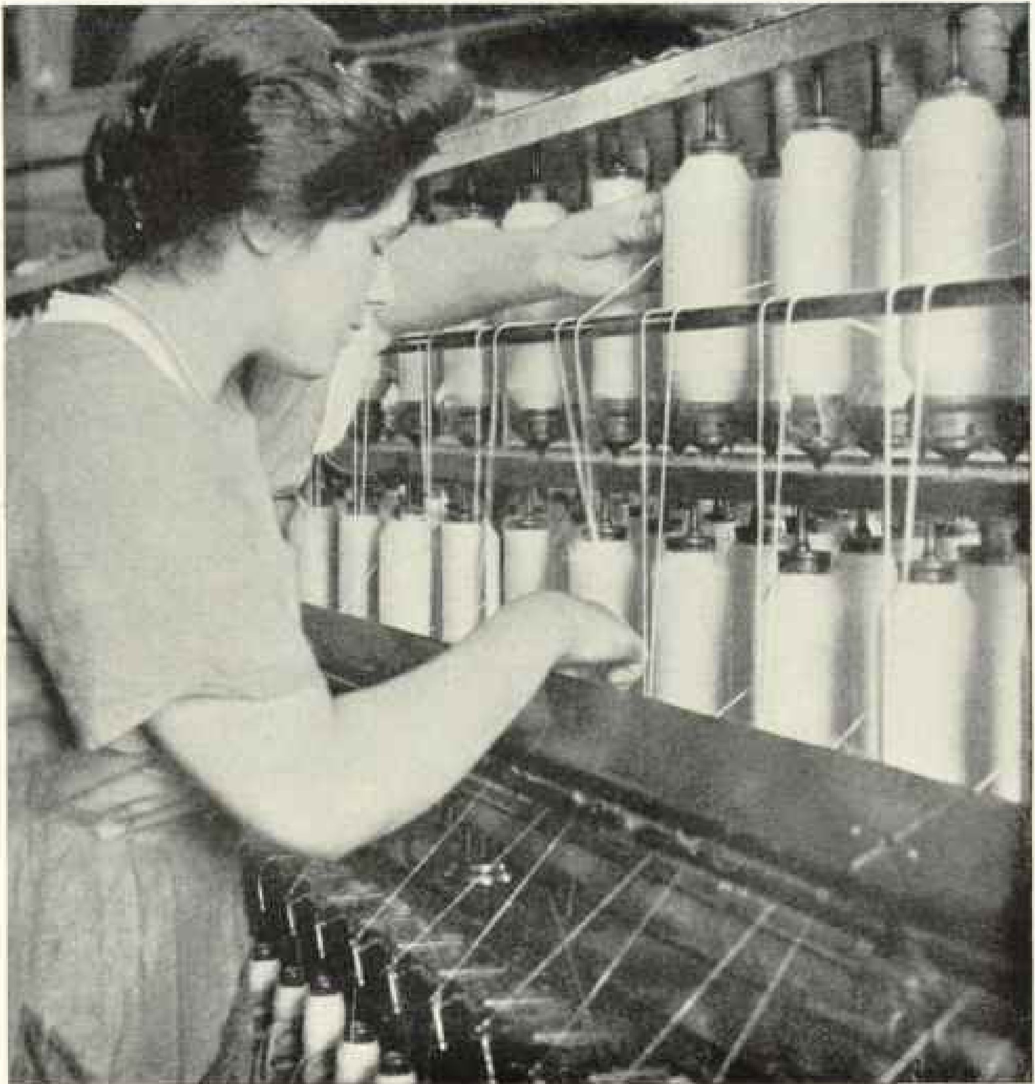
A COTTON-SPINNER KEEPING THE THREADS OF ROVING RUNNING PROPERLY FROM BOBBIN TO BOBBIN
