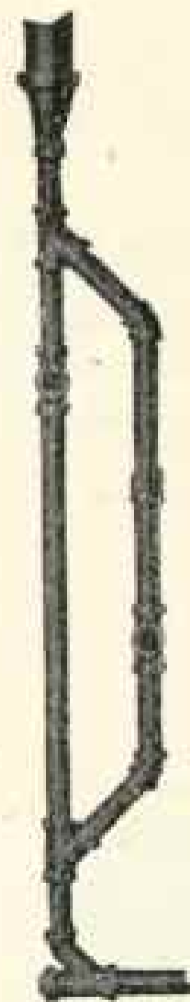
A typical Crane drainage pipe line showing the fittings ordinarily required in a 3-story dwelling. Pipes are shortened in the illustration because of limited space.
