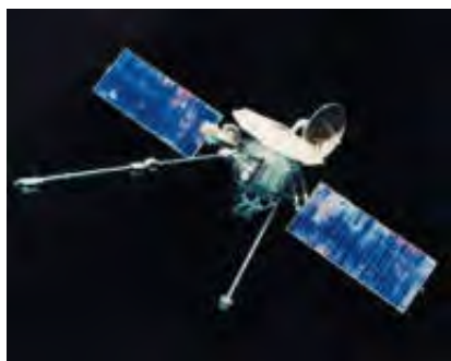
Mariner 10 space probe, which sent back to Earth valuable pictures and other data about Mercury.
