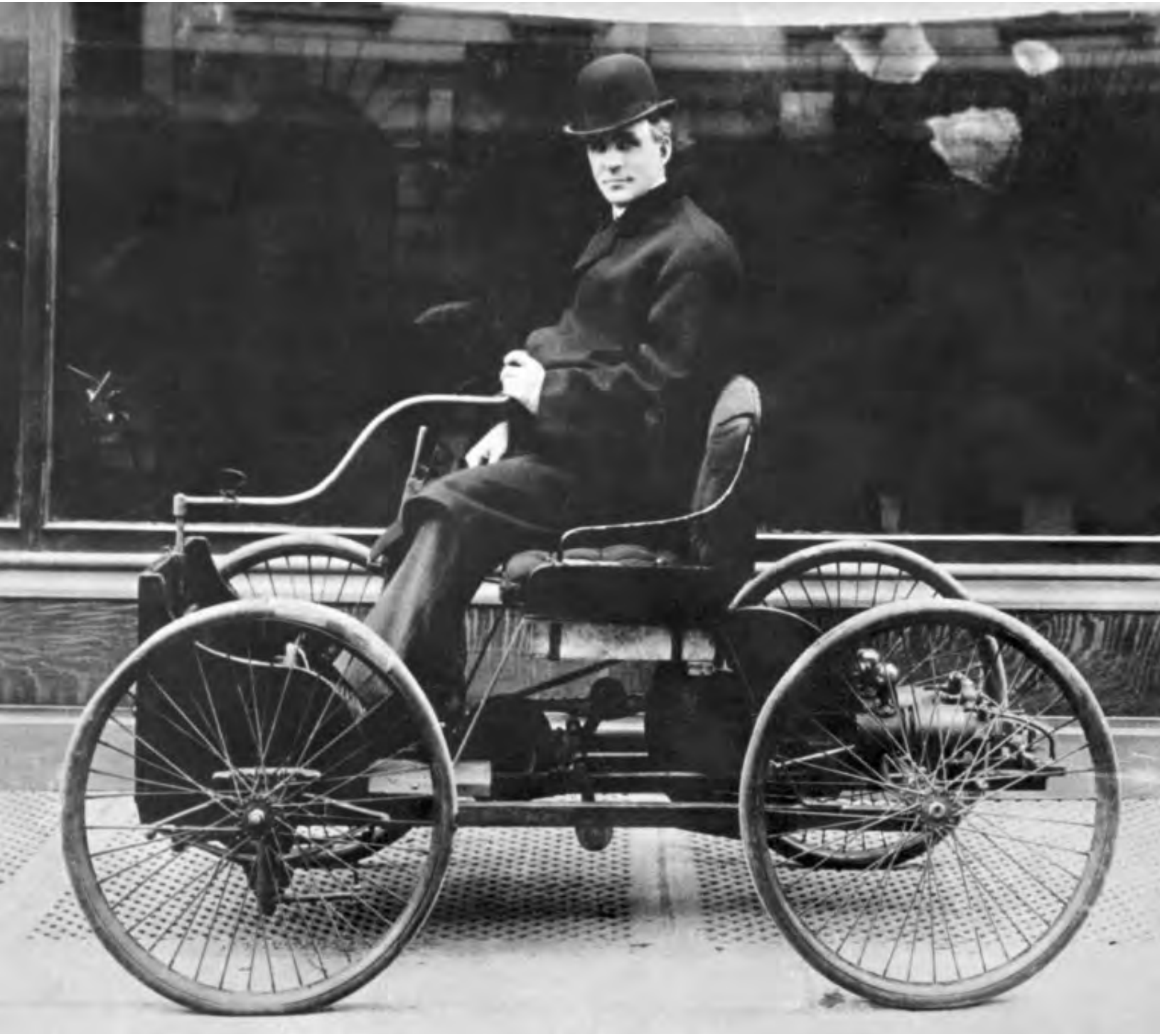
Henry Ford's first car was the Quadricycle, seen here with Ford driving. It had only two forward speeds and could not back up.
