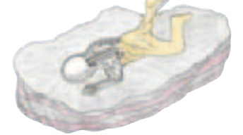
Cavity is filled with wet plaster of Paris
