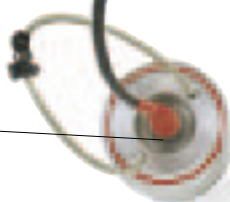
Yellow one-way electrode picks up vibrations
