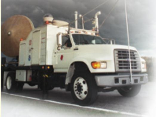
RADAR TRUCK USED BY STORM TRACKERS
