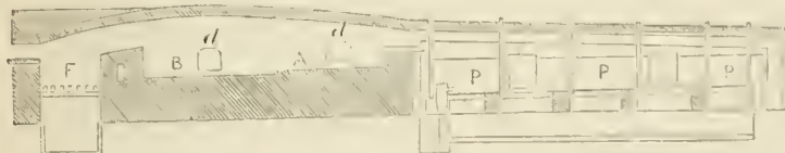
Fig. 4.—Section of Balling Furnace, shewing an evaporating pan for Soda-lye in connection with it.
