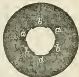
Fig. 3.—Section of the Enfield Rifle. a, groove; b, land.
