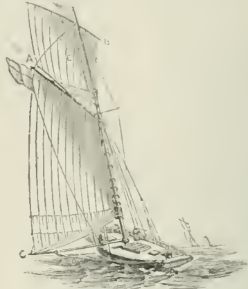
A, Gaff; B, Gaff-topsail-yard; C, Boom; D, Sheet; E, Gaff-topsail.
