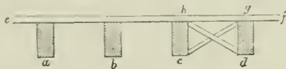
a, b, c, d , the joists; e, f , the flooring-boards; cg and dh , herring-bone strutting.
