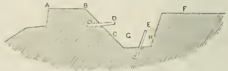
Fig. 1.—Fraise and Stockade (in section): AB, parapet; C, escarp; D, fraise; E, stockade; F, glacis; G, ditch; H, coulerscarp.
