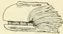
FIG. 39.—What a book may do if the back is not properly rounded.
