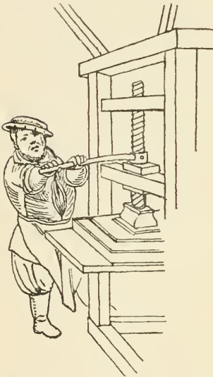
FIG. 68. — Printing press of about 1600. From Stradanus.
