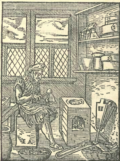
Type-Casting as Practised in 1564. [From Jost Amman.]
