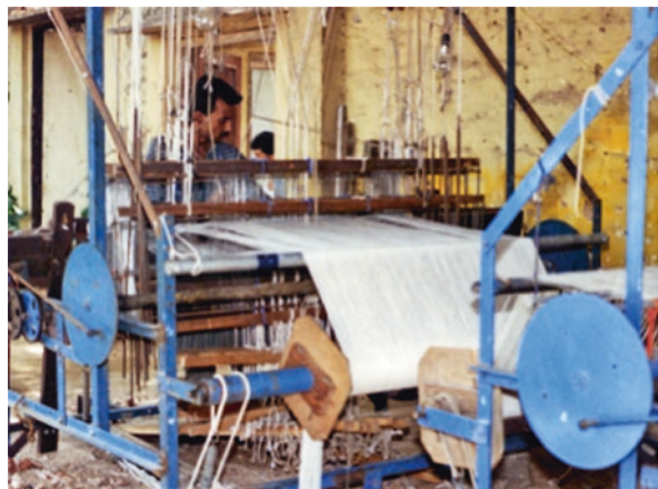
Fig. 3.2 The TARA 'Flying Shuttle Loom' – the powerloom without power: gives a weaver 3–4 times the income compared with a traditional loom (Photo: Development Alternatives)
