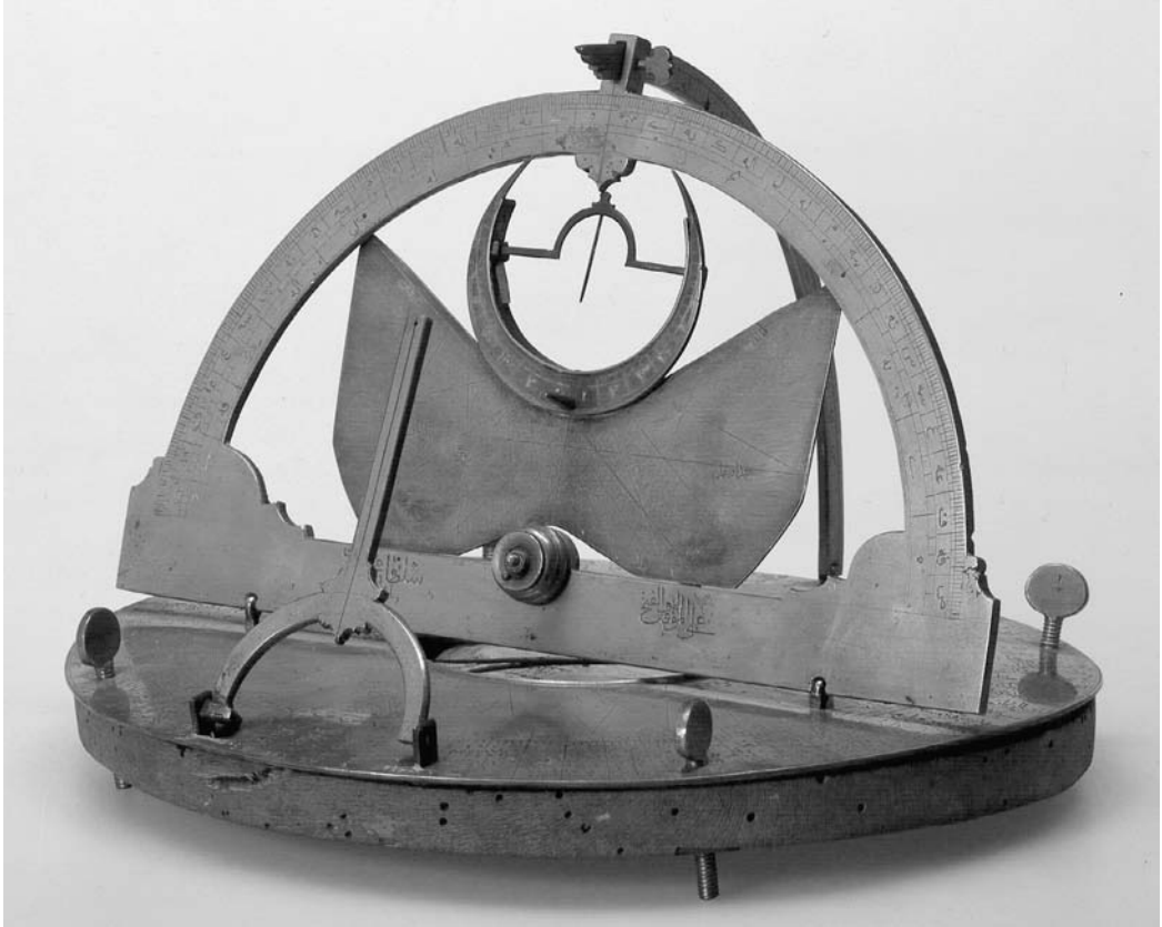
[iv] Qibla compass and sundial, open: Istanbul, 1161/1748. This complex device, termed an “equatorial circle” ( dā'irat al-mu'addil ) by its ninth/fifteenth century Egyptian inventor, combines a qibla compass with a sundial. Courtesy of the Nasser D. Khalili Collection, London (SCI 270).
