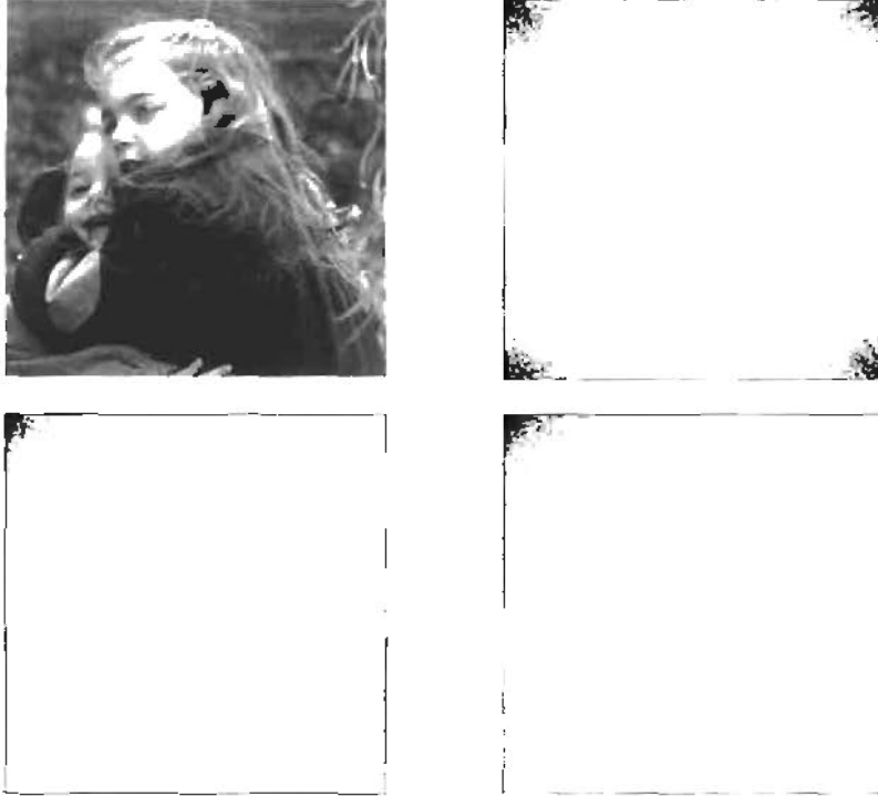
FIGURE 6.3: Example of an image and its magnitude DFT, DST, and DCT transforms, shown from top left to bottom left in the clockwise sense.
