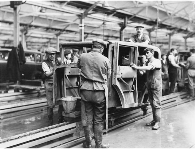
4. Mass production at Morris Motors, Cowley, Oxford, 1929. Here the body foundation is being rubbed down after the first coat of paint. The car industry, pioneered by William Morris at Cowley and Herbert Austin at Longbridge, made a dramatic impact on British economic life and leisure patterns in the twenties
