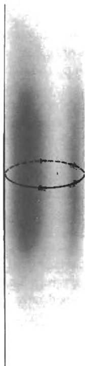
FIGURE A.14 Gaussian curvature of a cylinder is zero.
