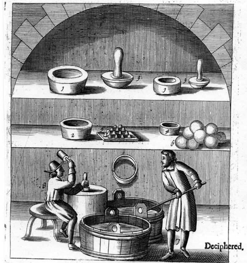
**FIGURE 26.** ■ Manufacture of cupels (using a paste made from crushed bone and beer) from Pettus' 1683 *Fleta Minor*. Compare this figure with the corresponding one (Figure 9) in the 1736 edition (i.e., the original 1574 edition), and you will note that costumes have been updated by a century while the apparatus remains unchanged.
