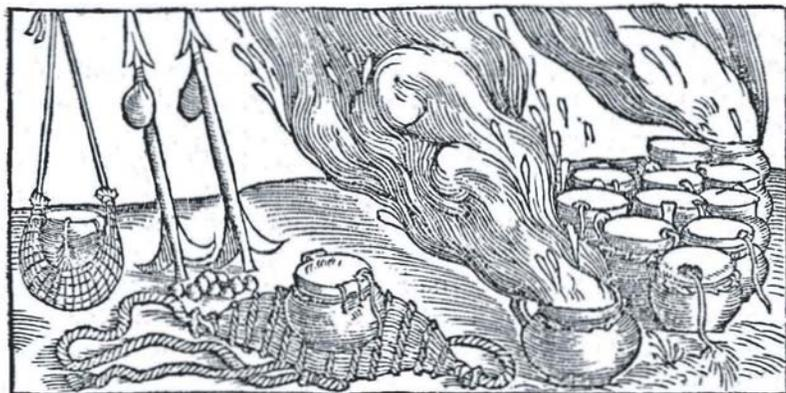
**FIGURE 33.** ■ Nasty munitions made from clay pots filled with coarse gunpowder, pitch, and sulfur, and sealed with congealed pig fat mixed with powder depicted in Biringuccio’s *Pirotechnia*. These are manufactured to be lighted and launched with malice using a sling. (From The Roy G. Neville Historical Chemical Library, a collection in the Othmer Library, CHF.)
