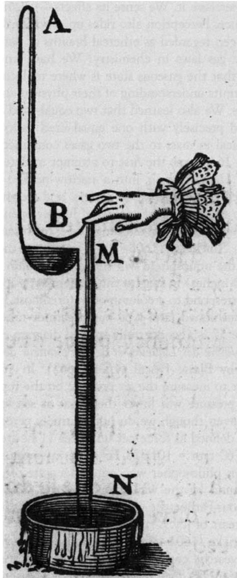
**FIGURE 143.** ■ A figure from Blaise Pascal's *Traitez de l'Equilibre des Liqueurs, et de La Pesanteur de La Masse de L'Air* (Paris, 1663) depicting a highly stylized barometer. He sent his brother-in-law Perier to measure the atmospheric pressure on a mountain top (courtesy Edgar Fahs Smith Collection, Rare Book and Manuscript Library, University of Pennsylvania).
