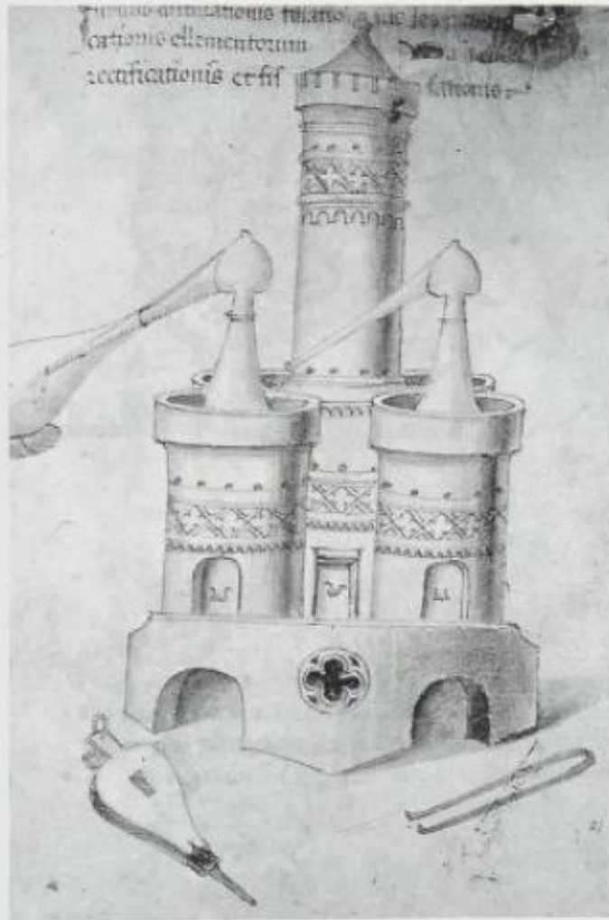
An alchemical furnace built in the form of a castle. The words at the top explain what it was used for: furnace for distillation, fixation, separation and rectification of the elements (15th century miniature). The alchemists called their furnace an athanor .
