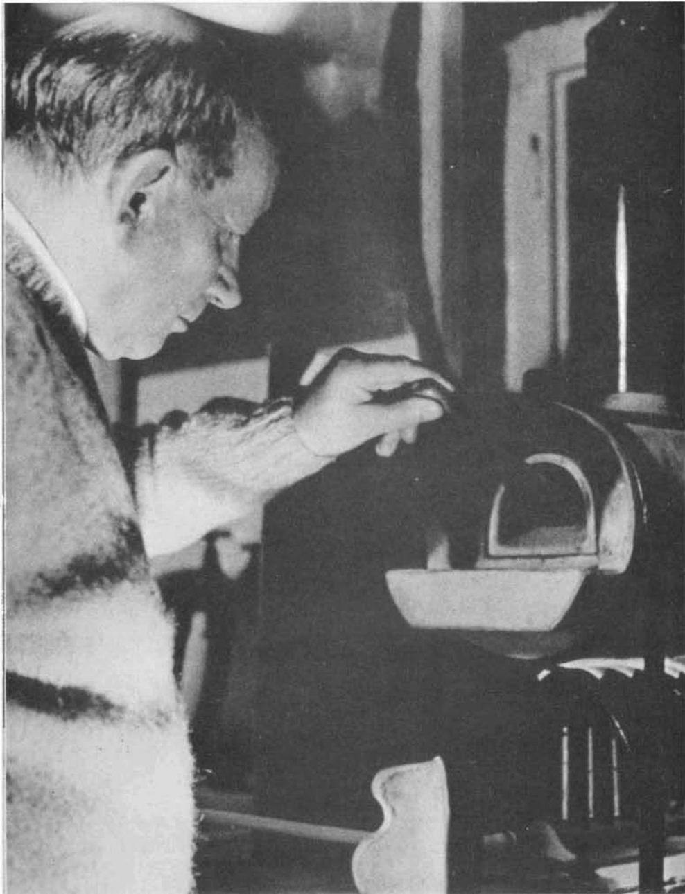
Incineration. Once the peat is fully dried out it is freed from any remaining deposits of carbon by incinerating it in an oven at a temperature of between 700 and 800°C. This operation takes several hours. Thus are obtained the ashes containing the vegetable salts.
