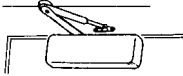
FIGURE 11.77 Door-closer spring closes the door, while a hydraulic mechanism (cylinder with piston) keeps the door from slamming.
