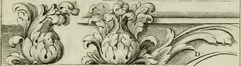
Rose of the Abacus of the Capital view'd Sidewise, and in Front.
