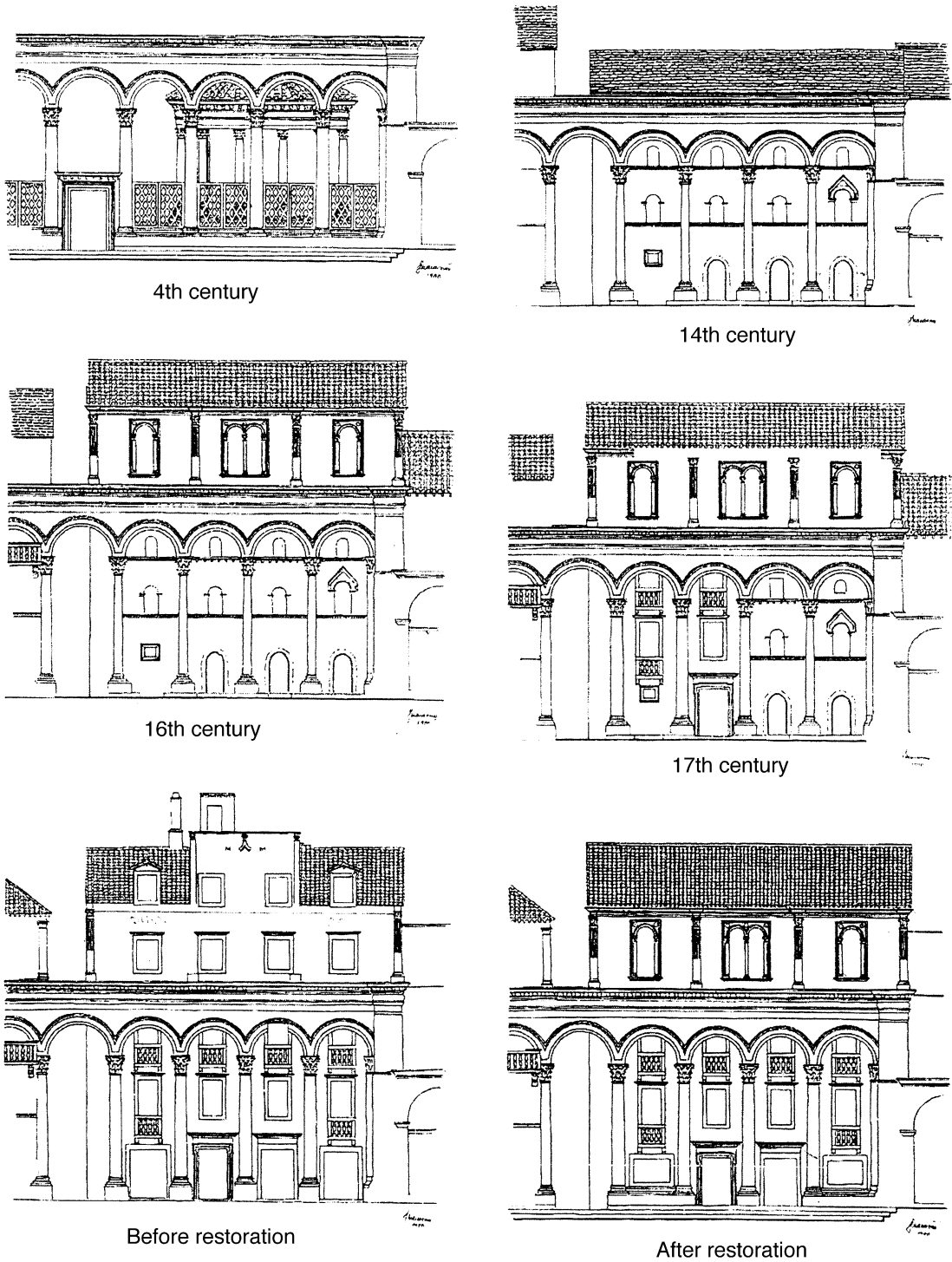
Figure 10.5 Historic phases in the transformation of the house of Cipci in the Peristyle of Diocletian's Palace in Split. The last phase shows the restoration of the house in the 1980s. (Drawing by J. Marasovic)
