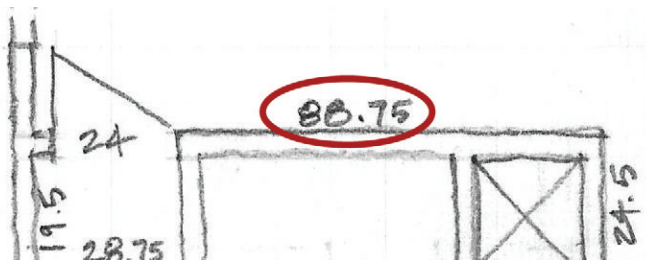
Figure 17.12 Record your measurements in decimal inches.
