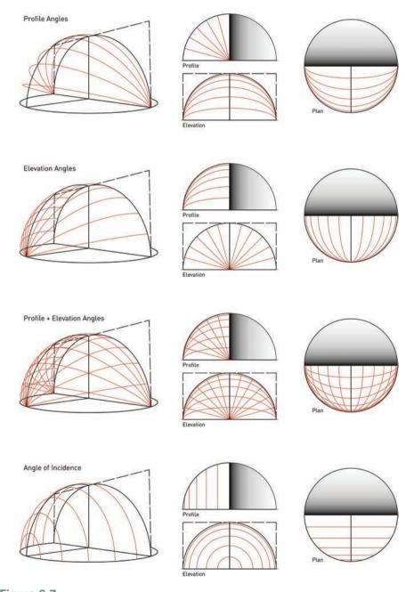
Figure 6.7 Surface Coordinate Transformations on the Sky Dome
