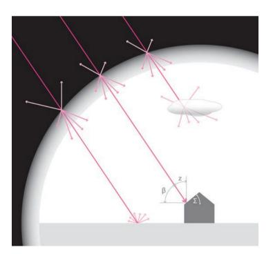
Figure 4.10 Interaction of Solar Radiation and the Atmosphere Greg Arcangeli
