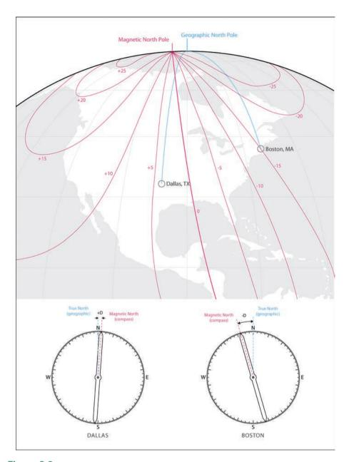
Figure 2.9 **Adjusting for Magnetic Declination**
