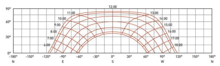
Figure 3.18 Modified Cylindrical Projection of the Sun Path for Austin, Texas Greg Arcangeli/Dason Whitsett
