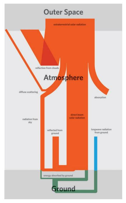
Figure 4.11 **Solar Radiation Flows** Greg Arcangeli
