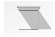
Figure 8.11 Importance of Elevation Angle in Shading Design
