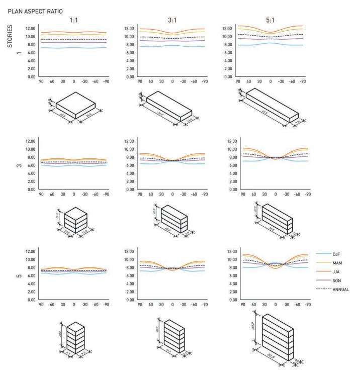
**Figure 5.7** Insolation on a Building by Orientation, Plan Aspect Ratio, and Height.
