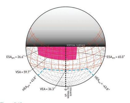
Figure 8.12 **Shading Mask for Specific Shading Criteria (Not Infinite)**
