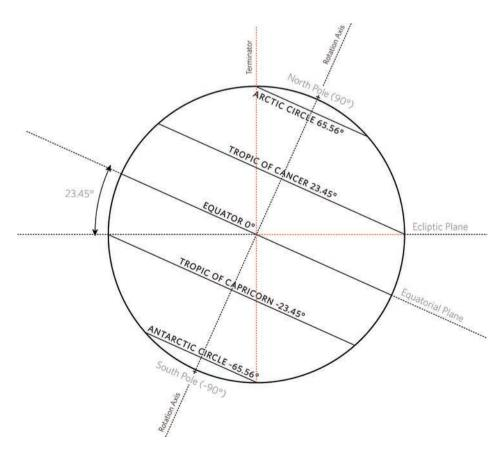
Figure 2.10 Geometry of the Earth and the ecliptic plane Greg Arcangeli
