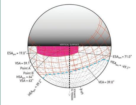
Figure 8.16 **Shading Mask for Example 8.2**
