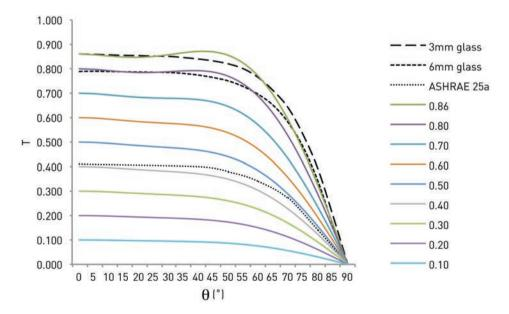
Figure 9.2 Transmittance Value by Angle of Incidence
