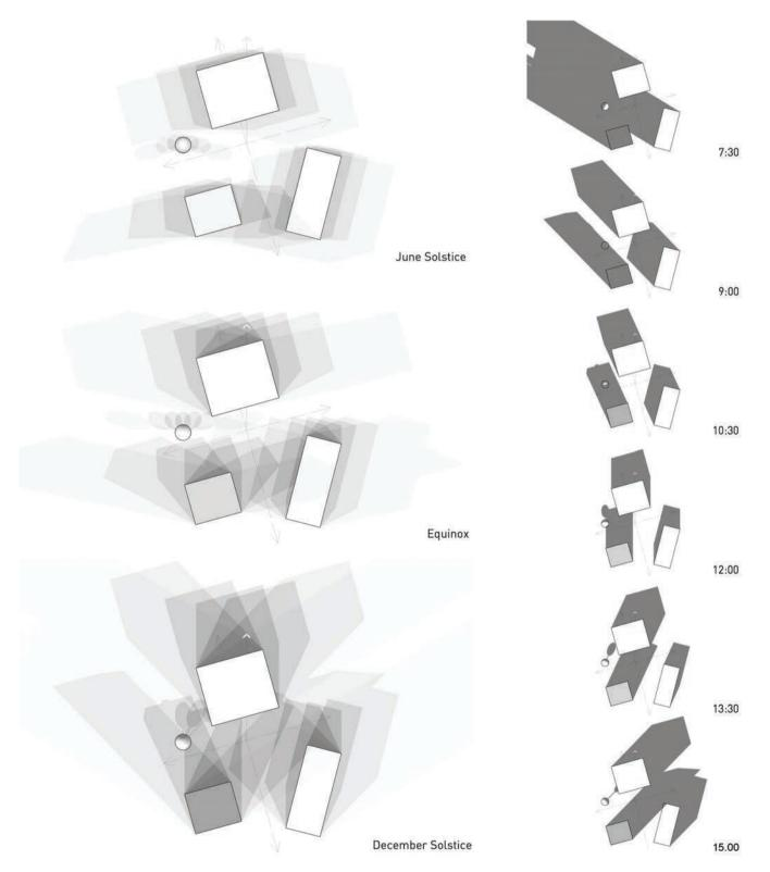
Figure 7.2 Composite Shadow Study Composite shadow analysis for building site shown in Figure 7.1. Dason Whitsett
