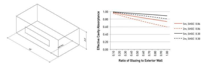
Figure 9.3 **Example Cavity Absorptance**
