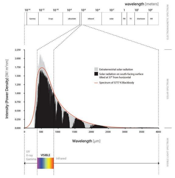
Figure 4.8 The Solar Radiation Spectrum Greg Arcangeli
