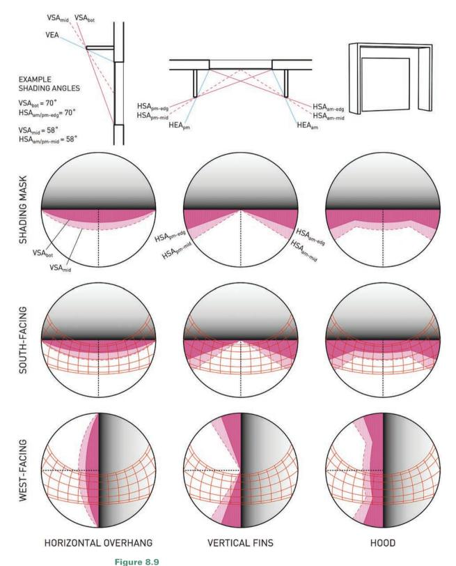
**Shading Masks for Common Shading Geometries**
