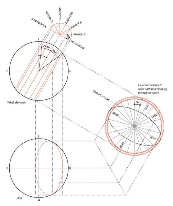
Figure 3.13 Construction of a Spherical Sun-Path Projection
