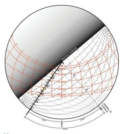
Figure 7.9 Equidistant Solar Protractor  $L = 30^{\circ}$ —Profile and Elevation Angles
