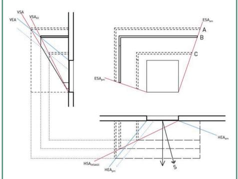
Figure 8.17 Solar Control Design for Surface of Arbitrary Orientation - Example 8.2 Dason Whitsett
