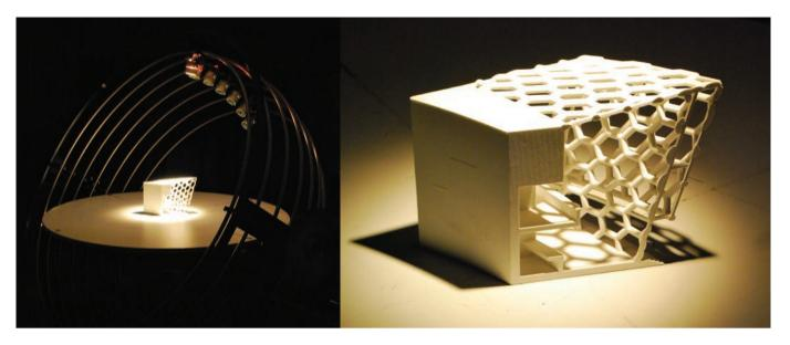
Figure 3.3 Heliodon in Use Testing a Model
