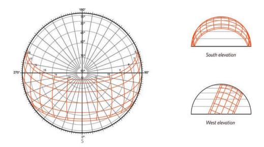
Figure 3.12 30° North Spherical Sun Path
