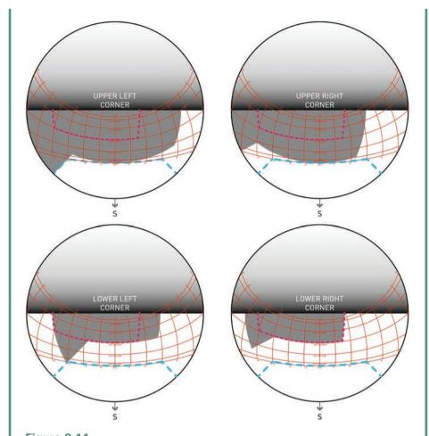
Figure 8.14 Sky-Dome Projection of Shading Device Design (at Four Corners)
