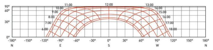
Figure 3.17 Cylindrical Projection of the Sun Path for Austin, Texas Greg Arcangeli/Dason Whitsett
