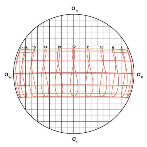
Figure 3.14 Spherical Sun-Path Projection with Cartesian Grid, Nairobi, Kenya Either polar or Cartesian coordinates may be used for the coordinate grid. Greg Arcangeli
