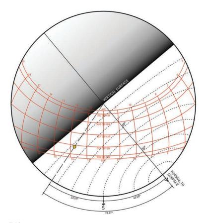
Figure 7.10 Equidistant Solar Protractor  $L = 30^{\circ}$  - Angle of Incidence
