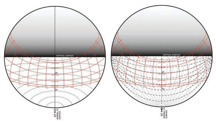
Figure 8.6 Solar Protractor for South-Facing Surface at 30° N Latitude - Angle of Incidence and Profile/ **Elevation Angles** Dason Whitsett
