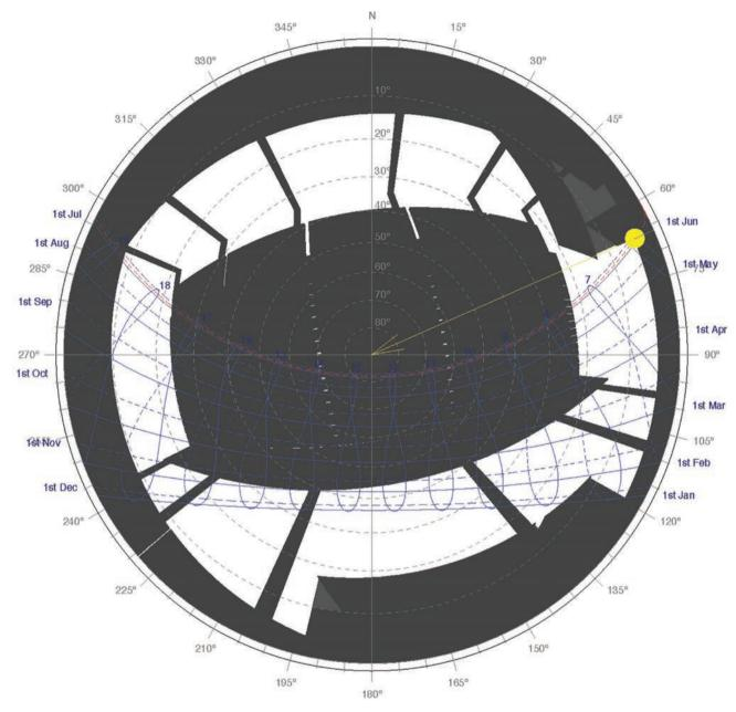
Figure 7.13 Sky Dome Projection of an Open Pergola Pollen Architecture and Design
