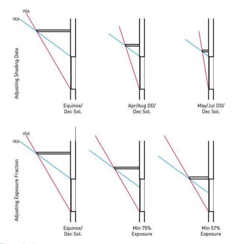
Figure 8.15 **Overhang Proportions for South-Facing Surface** Dason Whitsett
