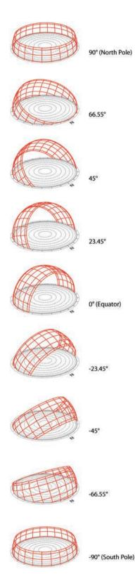
Figure 3.4 **Solar Path Band for Various Latitudes** Greg Arcangeli
