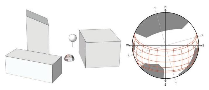
Figure 7.12 Completed Sky Dome Projection of a Site Dason Whitsett
