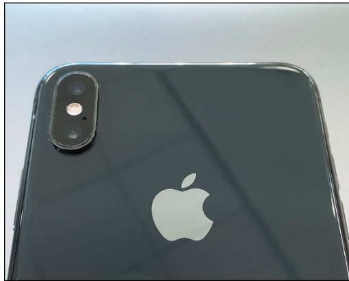
FIGURE 1-2: The dual lens iPhone XS Max's wide-angle and telephoto lenses.
