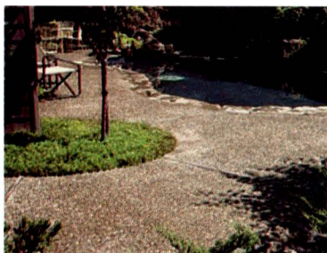
Exposed aggregate finish, broken by expansion joints, allows freeform.
