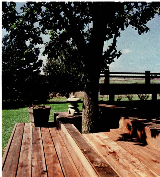
Cutouts in the decking allow trees to grow through and cover part of the deck. Care must be taken to allow a big enough hole for growth and wind sway. Never attach a deck directly to a tree, unless it's a tree house deck and is unattached to anything else.
