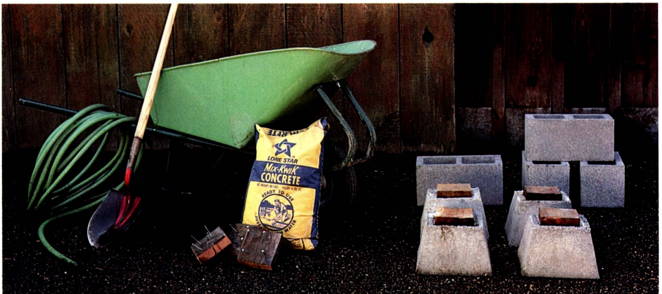
Tools and supplies for the do-it-yourself cement mixer include: wheelbarrow, shovel, hose and water, bucket, redwood nailing blocks, pre-cast piers and hollow-core concrete blocks.
