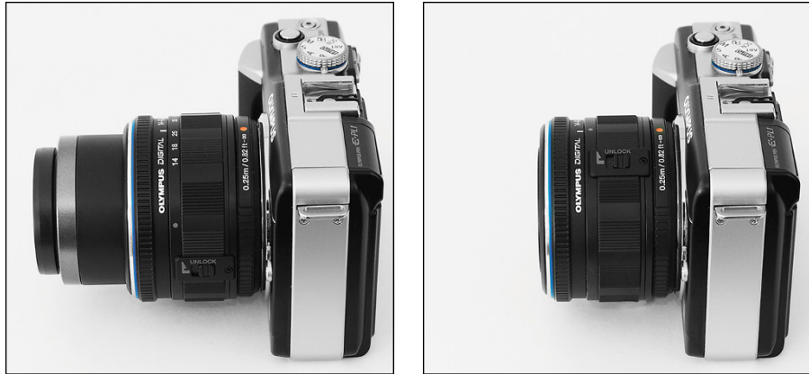
FIGURE 1-11: Some lenses collapse when not in use, taking up less room in your camera bag.
