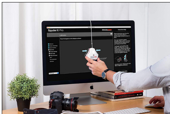
FIGURE 14-9: Monitor calibration tools such as this one from Datacolor ensure a more accurate display of your images.
