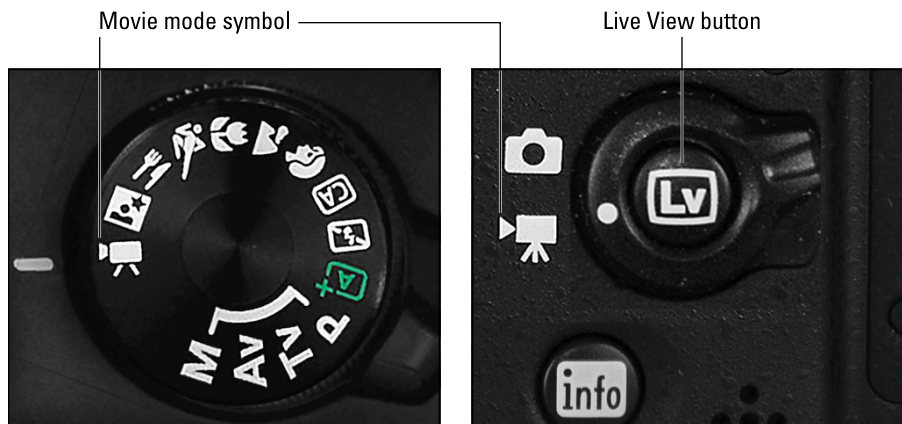
FIGURE 3-8: The control that sets the camera to movie mode usually looks like an old-fashioned movie camera.
