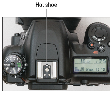
FIGURE 6-5: On most cameras, you connect an external flash via this connection, known as a hot shoe.
