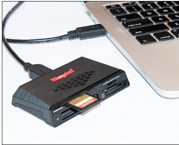
FIGURE 12-7: This card reader from Kingston works with types of camera memory cards.
