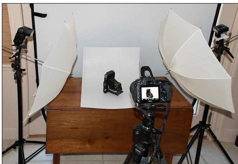
FIGURE 6-18: Here's a basic cross-lighting setup, which can produce shadow-free product shots.
