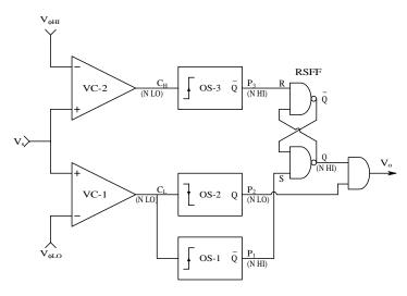
A nerve spike pulse-height window that produces an output pulse *only if* an input spike rises to its peak inside the window and then falls below the lower "sill." No output pulse is produced if an input spike rises through the window and exceeds the upper level, then falls below the sill.
