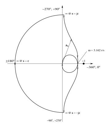
**FIGURE 5.13** The Nyquist vector contour plot of the NFB  $\mathbf{A}_L(\mathbf{s})$  of Equation 5.30. This  $\mathbf{A}_L(\mathbf{s})$  has a pole at the origin.
