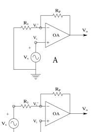
(A) An op amp connected as a noninverting amplifier. (B) An op amp connected as an inverting amplifier.
