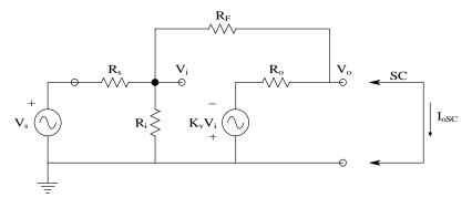
**FIGURE 4.2** Schematic of a simple Thevenin VCVS with negative feedback. See text for analysis.
