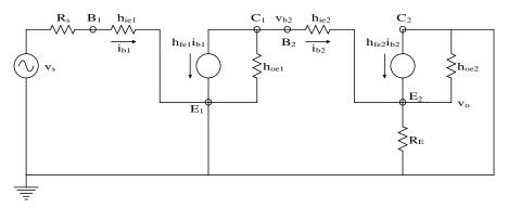
Top: feedback pair amplifier with load resistor in  $Q_2$ 's emitter. Bottom: MFSSM of the amplifier shown above. Analysis in text shows this amplifier has a high inverting mid-frequency gain; it does not emulate an emitter follower.
