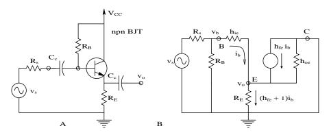
**FIGURE 2.17** (A) Schematic of a simple, capacitively coupled, emitter-follower amplifier. (B) MFSSM of the
