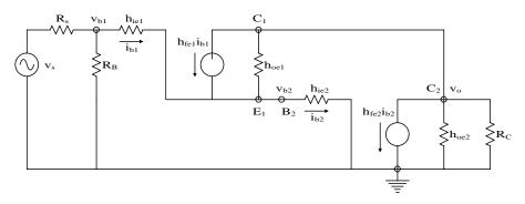
Top: a common-emitter Darlington amplifier. Bottom: *C–E h*-parameter MFSSM of the Darlington amplifier. Analysis is in the text.
