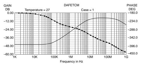
**FIGURE 3.9** Common-mode frequency response of the JFET DA of Figure 3.7A. Note that the AR rises +3 dB from -46 dB at 110 kHz, then rises to a maximum of -7 dB and falls off again by 3 dB at approximately 400 MHz. Phase is bold trace with squares.
