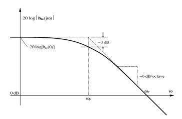
**FIGURE 2.42** Bode frequency response magnitude of  $|h_{f_k}(j\mathbf{w})|$ .
