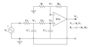
**FIGURE 7.1** A Sallen and Key quadratic low-pass filter.
