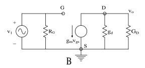
(A) An n-channel JFET "grounded-source" amplifier.  $C_S$  bypasses small ac signals at the JFET's source to ground, making  $v_s = 0$ . (B) MFSSM of the amplifier. The same MFSSM would obtain if a p-channel JFET were used.
