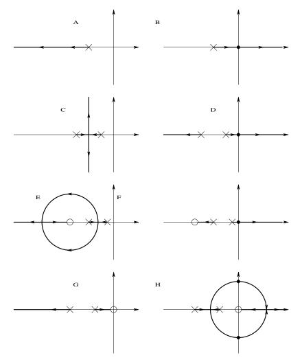
(A) through (L): Representative root-locus plots for six loop gain configurations for NFB and PFB conditions. PFB root-locus plots are on the right.
