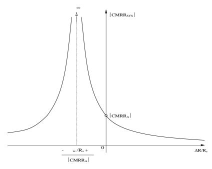
**FIGURE 3.14** The CMRR of a balanced input DA as a function of the incremental change in one input (Thevenin) resistance. Note that a critical value of  $\Delta R/R_s$  exists that theoretically gives infinite CMRR.
