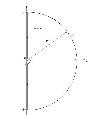
**FIGURE 5.6** The contour  $C_1$  containing **s** values traversed clockwise in the s-plane.
