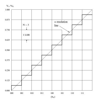
**FIGURE 10.7** I/O characteristic of an ideal 3-bit DAC.
