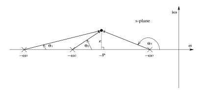
s-Plane vector diagram illustrating the vectors and angles required in calculating the breakaway point of complex conjugate locus branches when they leave the real axis. (See part 7 of the nine basic root-locus plotting rules in the text.)
