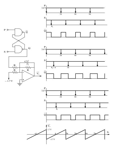
**FIGURE 12.8** The RS flip-flop PD and its waveforms. The bottom graph shows a plot of the (offset) average output voltage of this PD vs. the phase difference between TTL inputs P and S. Note the significant zeros are at odd integer multiples of  $\pi$ .
