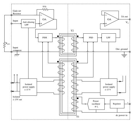
**FIGURE 8.3** Simplified schematic of an Analog Device's AD289 magnetically isolated isolation amplifier (IsoA). An AD620 IA is used as a differential front end for the IsoA; it is powered from the AD289's isolated power supply.
