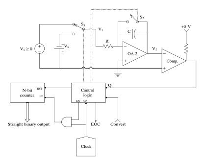
**FIGURE 10.15** Block diagram of a unipolar-input dual-slope integrating ADC.
