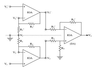
**FIGURE 8.2** The three-op amp instrumentation amplifier.
