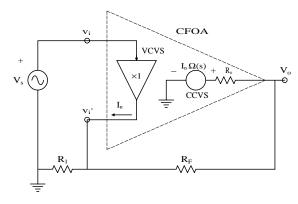
**FIGURE 6.5**Simplified internal circuitry of a current-feedback op amp. The output current of the unity-gain VCVS controls the output of the Thevenin CCVS.
