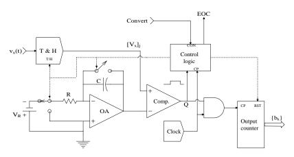
**FIGURE 10.14** Block diagram of a single-slope integrating ADC.
