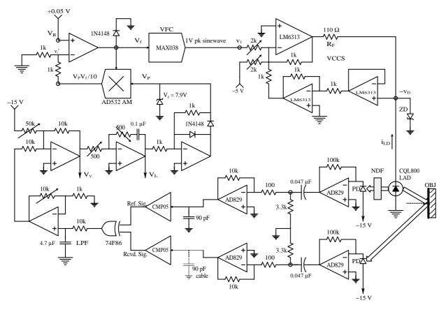
**FIGURE 12.48** Simplified schematic of the LAVERA system showing the ubiquitous use of op amps.
