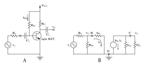
(A) Schematic of a simple, capacitively coupled, grounded-emitter BJT amplifier. (B) Linear, mid-frequency, small-signal model (MFSSM) of the grounded-emitter amplifier. Note that, at mid-frequencies, capacitors are treated as short circuits and DC source voltages are small-signal grounds. The mid-frequency gain,  $v_{\rm o}/v_{\rm s}$ , can be found from the model; see text.
