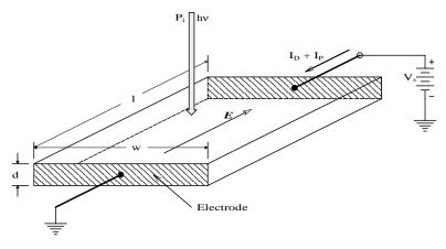
**FIGURE 2.67** Geometry of a photoconductor slab.
