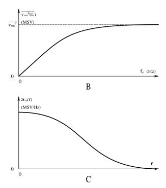
**FIGURE 9.1** (A) System for measuring the integral power spectrum (cumulative mean-squared noise characteristic) of a noise voltage source,  $e_N(f)$ . (B) Plot of a typical integral power spectrum. (C) Plot of a typical one-sided power density spectrum. See text for description.
