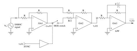
**FIGURE 11.13**Schematic of a three-op amp synchronous (phase-sensitive) rectifier used to demodulate a DSBSC-modulated carrier.
