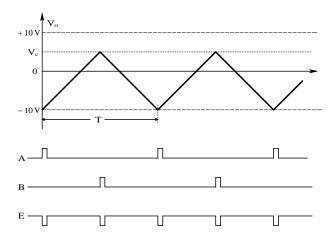
**FIGURE 12.22**Top: Schematic of a hybrid VPC with digital output. Bottom: Waveforms of the hybrid VPC.
