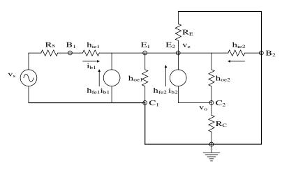
MFSSM for the EF-GB amplifier of Figure 2.19(C). See text for analysis.
