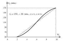
**FIGURE 12.20** Top: A VCO that uses the voltage-variable capacitance of two varactor diodes to set its output frequency. Bottom: The frequency vs. dc control voltage characteristic of the varactor VCO.
