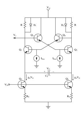
**FIGURE 12.17**Simplified schematic of a *v*oltage-*c*ontrolled, *e*mitter-*c*oupled, (astable) *m*ultivibrator (VCECM).
