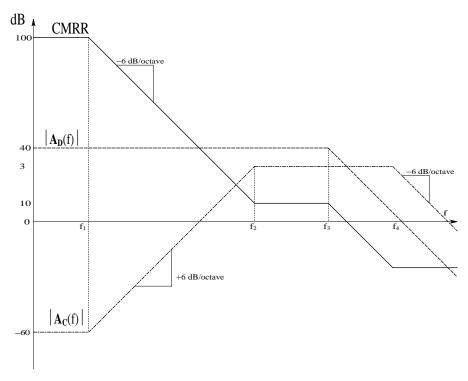
**FIGURE 3.4**Typical Bode plot asymptotes for the common-mode gain frequency response, the difference-mode gain frequency response, and the common-mode rejection ratio frequency response.
