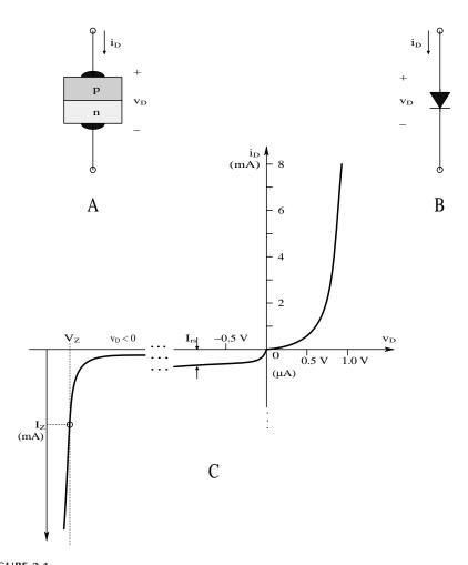
**FIGURE 2.1**(A) "Layer cake" cross section of a silicon *pn* junction diode. (B) Diode symbol. (C) Typical I–V
