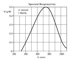
**FIGURE 2.66**Top: schematic of the Burr–Brown OPT202 IC photosensor. Bottom: spectral sensitivity of the OPT202 sensor. See text for details.
