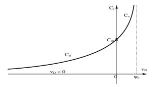
**FIGURE 2.4** How the equivalent junction capacitance of a pn diode varies with  $v_D$ .  $C_d$  is mostly depletion capacitance (see text) and  $C_s$  is due to stored minority carriers associated with forward conduction.
