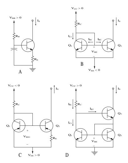
Four BJT circuits used for high-impedance current sources and sinks in the design of differential amplifiers and other analog ICs. They can serve as high-impedance active loads. (A) Collector of simple BJT with unbypassed emitter resistance. (B) Basic two-BJT current sink. (C) Widlar current source (*pnp* BJTs are used). (D) Wilson current sink.
