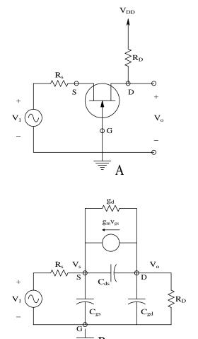
**FIGURE 2.49**(A) A JFET grounded-gate amplifier. (B) The HFSSM for the amplifier.
