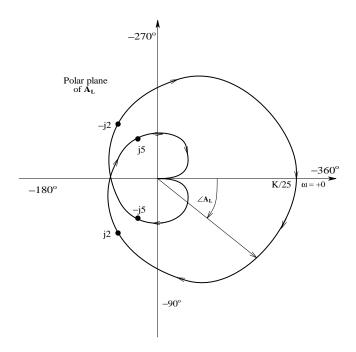
The Nyquist vector contour of the SISO negative feedback system's  $A_L(s)$  as s traverses  $C_1$ '. Note that this type of contour is always symmetrical around the real axis, and is closed because  $C_1$ ' is also closed. See text for discussion of stability.
