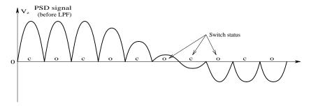
**FIGURE 11.14**Waveforms relevant to the operation of the synchronous rectifier of Figure 11.13. Top: Modulating signal. Middle: DSBSC signal. Bottom: Detected signal before LPF.
