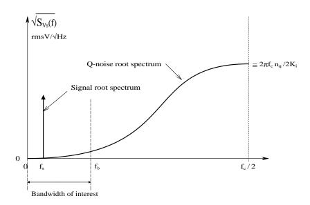
**FIGURE 10.25** A typical root power density spectrum of signal and quantization noise in a first-order  $\Delta$ – $\Sigma$
