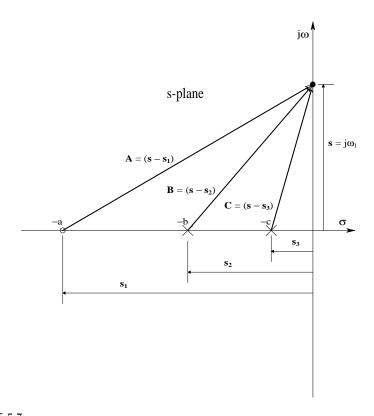
**FIGURE 5.7** The s-plane showing vector differences from the real zero and two real poles of a low-pass filter to  $\mathbf{s} = j\omega_1$ .
