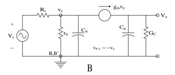
(A) A BJT grounded-base amplifier. (B) The HFSSM for the amplifier. Note that the model does not have a Miller feedback capacitor.
