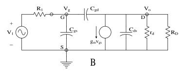
**FIGURE 2.48**(A) A JFET grounded-source amplifier. (B) The HFSSM for the amplifier.
