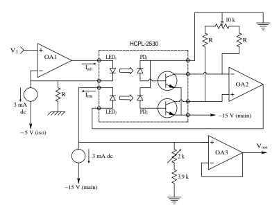
A linear analog photo-optic coupler used to provide galvanic isolation between the battery-operated ECG measurement differential amplifier and band-pass filter, and the output recording and display systems.
