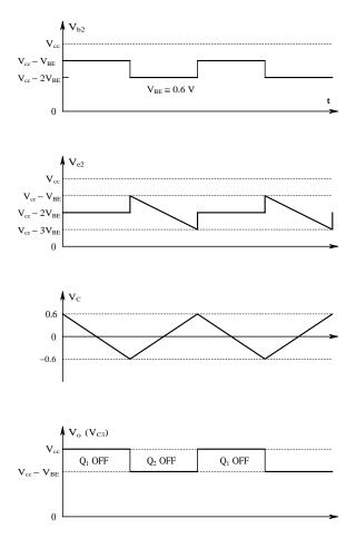
**FIGURE 12.19**Relevant waveforms in the VCECM for two cycles of oscillation.
