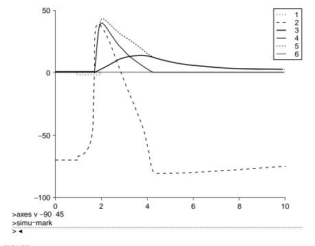
**FIGURE 1.1** Results of a Simnon<sup>TM</sup> simulation of the Hodgkin–Huxley 1952 mathematical model for nerve action potential generation. Traces: (1)  $J_{in}$  ( $\mu$ A/cm²). (2)  $v_m$ (t) (transmembrane potential). (3)  $g_K$ (t,  $v_m$ ) mS/cm². (4)  $g_{Na}$ (t,  $v_m$ ) mS/cm². (5)  $g_{net} = g_K + g_{Na} + gL$  mS/cm². (6)  $J_{in}$ ,  $\mu$ A/cm². (Northrop, R.B. 2001. *Introduction to Dynamic Modeling of Neuro-Sensory Systems*. CRC Press, Boca Raton, FL.)
