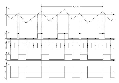
**FIGURE 10.22** Waveforms in a first-order  $\Delta$ – $\Sigma$  modulator when  $V_x = +V_R/4$ .
