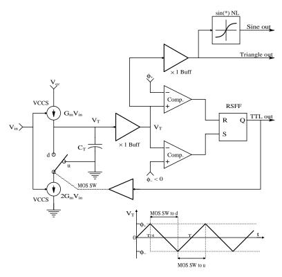
**FIGURE 12.16**Block diagram of a switched integrating capacitor VCO.
