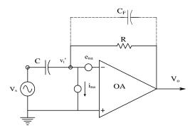
Circuit for an op amp differentiator. In this problem, the op amp's frequency response is considered, as well as its short-circuit input voltage noise root power spectrum, and input current noise root spectrum.
