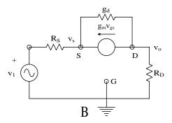
(A) An n-channel MOSFET grounded-gate amplifier. (B) MFSSM of the MOSFET G-G amplifier. See text for analysis.
