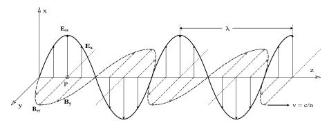
**FIGURE 12.37** Diagram of a linearly polarized electromagnetic wave (e.g., light) propagating in the **z** direction.  $\mathbf{B}_{\mathbf{v}}(t)$  is orthogonal in space to  $\mathbf{E}_{\mathbf{v}}(t)$ .
