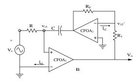
(A) A CFOA connected as a conventional integrator. The circuit does not work. (B) Two CFOAs connected to make a near ideal inverting integrator.
