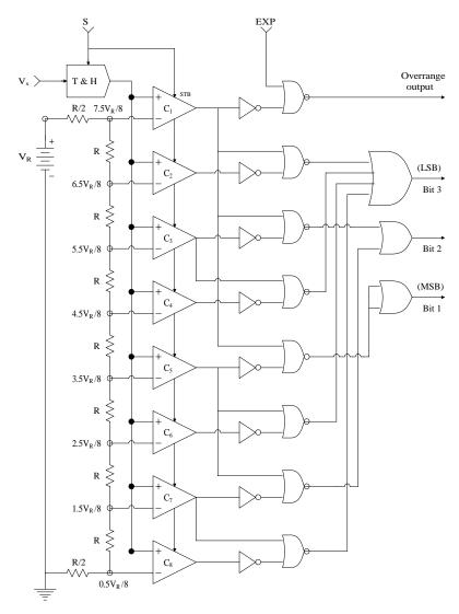
FIGURE 10.17 A 3-bit flash ADC.
