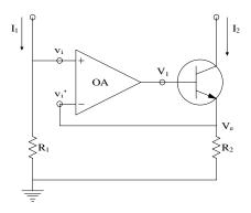
4.7 The op amp circuit shown in Figure P4.7 is a form of current mirror. The BJT can be modeled by its MFSSM with  $h_{re} = h_{oe} = 0$ . The op amp is ideal except for the gain:
