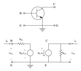
Top: an *npn* BJT viewed as a two-port circuit. Bottom: the linear, common-emitter, two-port, small-signal, *h*-parameter model for the BJT operating around some *Q* in its linear region. Note that the input circuit is a Thevenin model and the output is a Norton model.
