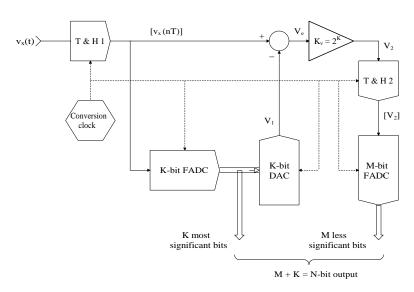
**FIGURE 10.19** Architecture of a two-step flash ADC. This design is more efficient when  $N \ge 8$  is desired.
