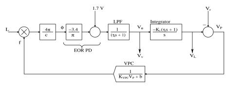
**FIGURE 12.47**Systems block diagram of the LAVERA system of Figure 12.45.
