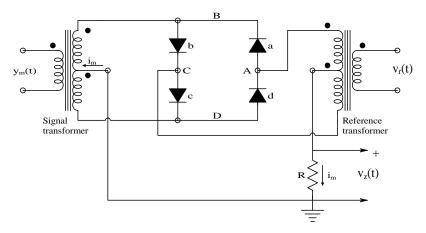
**FIGURE 12.2** A balanced-bridge diode PSR.
