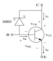
**FIGURE 2.8** Use of an SBD to make a Schottky transistor. The SBD prevents XS stored charge in the BJT's *C–B* junction.
