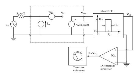
**FIGURE 9.11** A test circuit for measuring an amplifier's SNF.
