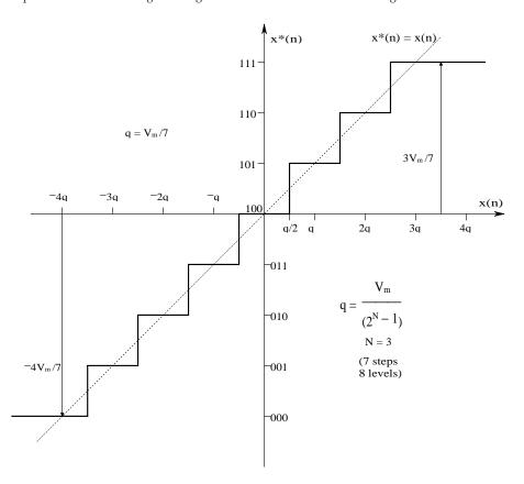
**FIGURE 10.27** A 3-bit rounding quantizer I/O function.
