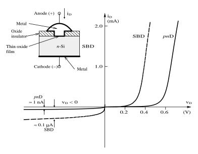
**FIGURE 2.6** The static I–V curves of a Schottky barrier diode and a pn junction diode.
