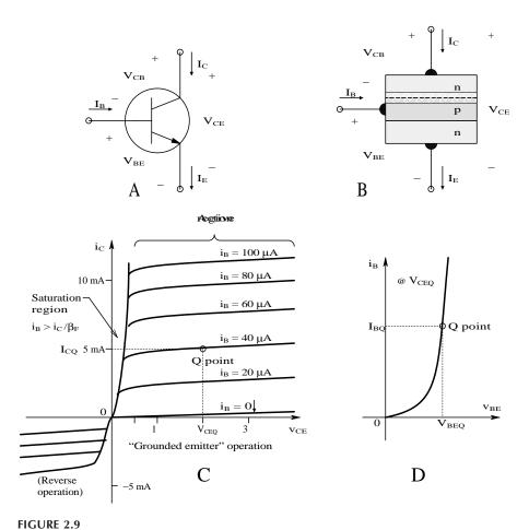
(A) Symbol for an npn BJT. (B) "Layer cake" cross section of a forward-biased npn BJT. The cross-hatched layer represents the depletion region of the normally reverse-biased C-B junction. (C) Collector–base I–V curves as a function of  $i_B$  for the *npn* BJT. (D) Base–emitter I–V curve at constant  $V_{CEO}$ . The B-E junction is normally forward biased.
