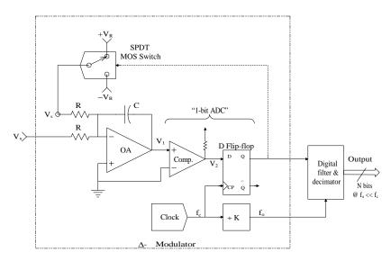
FIGURE 10.20 Block diagram of a first-order, delta–sigma ADC. The  $\Delta$ – $\Sigma$  modulator is in the dotted box.
