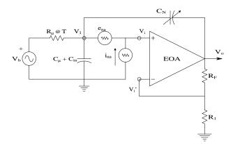
Schematic of a noninverting electrometer op amp with positive voltage feedback through a small neutralizing capacitor,  $C_N$ . This circuit is used with glass micropipette microelectrodes to increase system bandwidth.
