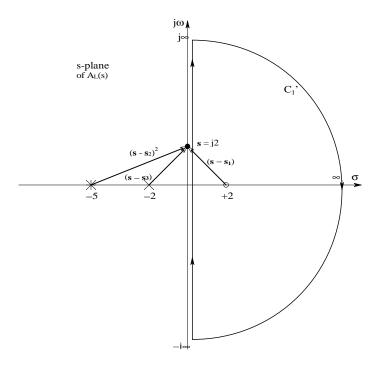
The vector s-plane of the loop gain showing vector differences and contour  $C_1'$  for a negative feedback system's  $A_L(s)$  having a real zero in the right-half s-plane. s traverses the contour clockwise.
