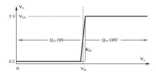
Top: analog comaparator. Bottom: transfer characteristic of the comparator. Comparator gain,  $K_D$ , in the linear region is as high as an op amp.
