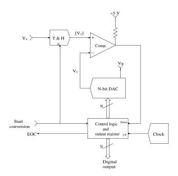
**FIGURE 10.12**Block diagram of the popular successive-approximation ADC.
