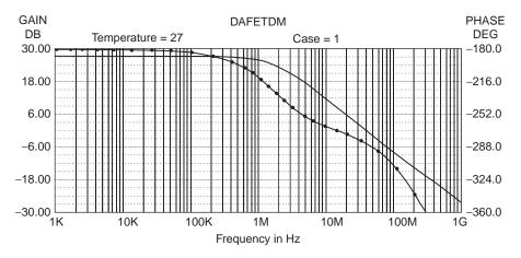
**FIGURE 3.8** Difference-mode frequency response of the JFET DA of Figure 3.7A. The –3-dB frequency is approximately 1.9 MHz. See text for details.
