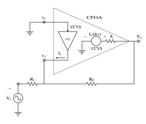
**FIGURE 6.6** A CFOA connected as an inverting amplifier.
