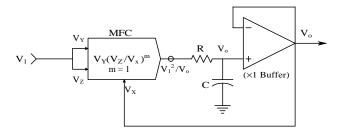
**FIGURE 12.31** A true RMS conversion circuit using a multifunction converter.
