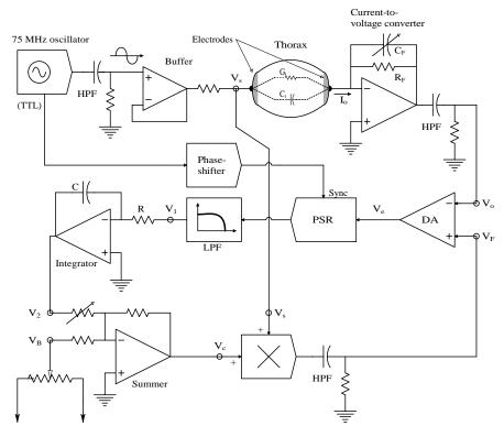
**FIGURE 12.49** Block diagram of the author's self-nulling admittance plethysmograph.
