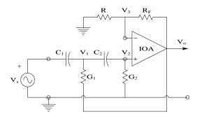
**FIGURE 7.3** A Sallen and Key quadratic high-pass filter.
