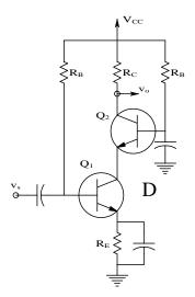
Four common two-BJT amplifier configurations: (A) The Darlington pair. Note that  $Q_1$ 's emitter is connected directly to  $Q_2$ 's base. (B) The feedback pair. The collector of the  $pnp\ Q_1$  is coupled directly to the  $npn\ Q_2$ 's base. (C) The emitter-follower–grounded-base (EF–GB) BJT pair. (D) The cascode pair.
