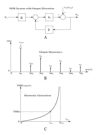
(A) Block diagram of a SISO negative voltage feedback system with output harmonic distortion voltage introduced in the last (power) stage. A sinusoidal input of frequency  $\omega_o$  is assumed. (B) Rms power spectrum of the feedback amplifier output.  $v_{os1}$  is the RMS amplitude of the fundamental frequency output. (C) Plot of how total harmonic distortion typically varies as a function of the amplitude of the fundamental output voltage.
