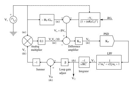
**FIGURE 12.50** Systems block diagram describing the dynamics of the self-nulling plethysmograph.
