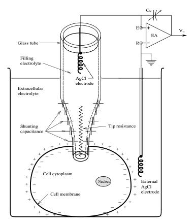
**FIGURE 1.6** Schematic cross section (not to scale) of an electrolyte-filled, glass micropipette electrode inserted into the cytoplasm of a cell. Ag AgCl electrodes are used to interface recording wires (generally Cu) with the electrolytes.
