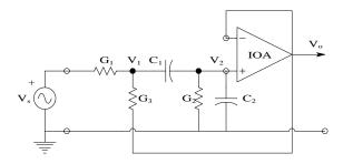
**FIGURE 7.4** A Sallen and Key quadratic band-pass filter.
