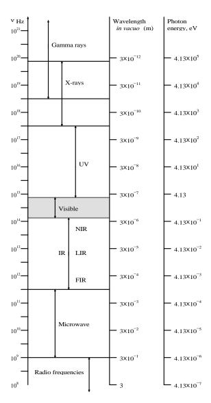
**FIGURE 2.55** The electromagnetic spectrum.
