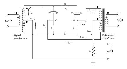
**FIGURE 12.3** The diode bridge PSR when diodes *a* and *b* are conducting, and *c* and *d* are blocking current flow.
