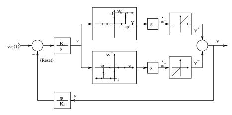
**FIGURE 11.9** Block diagram of a two-sided, integral pulse frequency modulation (IPFM) system.
