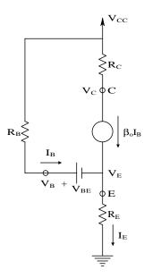
**FIGURE 2.12** Model for dc biasing of an *npn* BJT with collector, base, and emitter resistors. See text for analysis.
