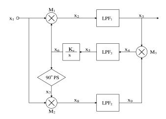
**FIGURE 11.15**Block diagram of a simple Costas PLL.
