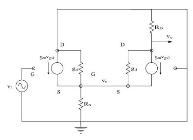
**FIGURE 2.37** MFSSM for the two-MOSFET SF/GG amplifier. See text for analysis.
