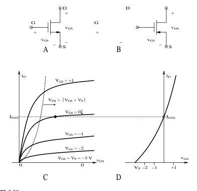
**FIGURE 2.30** (A) Symbol for an n-channel MOSFET. (B) Symbol for a p-channel MOSFET. (C) The  $i_D = f(v_{GS}, v_{DS})$  curves for an n-channel depletion MOSFET. (D) The  $i_D = f(v_{GS})$  curve for a saturated-channel, n-channel depletion MOSFET.
