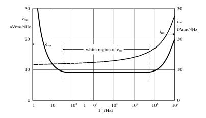
**FIGURE 9.6** Plots of the  $e_{na}$  and  $i_{na}$  root power density spectra vs. f for a typical low-noise FET headstage amplifier. Note that  $e_{...}$  has a low frequency  $1/\div f$  component and  $i_{...}$  does not.  $i_{...}$  and  $e_{...}$  increase
