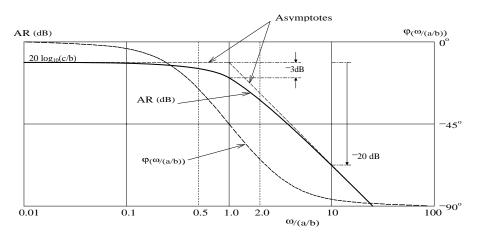
**FIGURE 5.1**Normalized Bode plot for a one real pole low-pass filter. Asymptotes, AR, and phase are shown.
