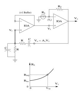
Top: schematic of a PFB Wien bridge oscillator. The buffer amp is not really necessary if a high input resistance op amp is used for the output. As in the case of the phase-shift oscillator, the oscillation amplitude is regulated by nonlinear feedback from a lamp. Bottom: the lamp's resistance as a function of the RMS voltage,  $V_1$ , across it.
