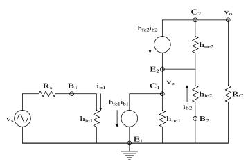
**FIGURE 2.24** MFSSM for the cascode amplifier of Figure 2.19(D). See text for analysis.
