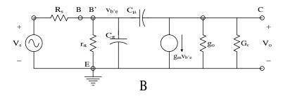
(A) A basic BJT "grounded-emitter" amplifier; the emitter is assumed to be at small-signal ground at mid- and high-frequencies. (B) Hybrid pi HFSSM for the amplifier. Note that  $C_m$  makes a Miller feedback path between the output node and the  $v_{be}$  node.
