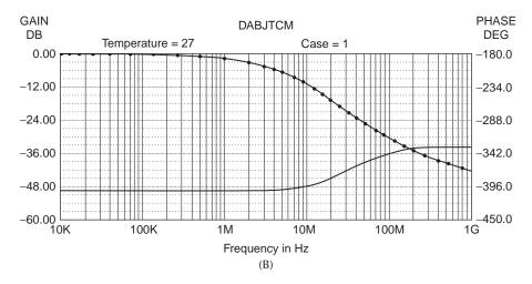
**FIGURE 3.10** Common-mode gain frequency response of the BJT DA of Figure 3.6A with various values of parasitic emitter capacitance,  $C_e$ , showing how  $C_e$  can improve the DA's CMRR by giving a low CM gain at high frequencies. (A) CM gain frequency response (FR) with  $C_e = 0$ . (B) CM gain
