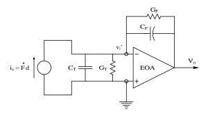
An electrometer op amp is used to make a charge amplifier to condition the output of a piezoelectric force transducer. See text for analysis.
