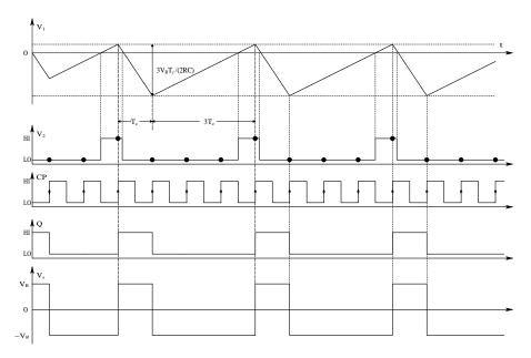
**FIGURE 10.23** Waveforms in a first-order  $\Delta$ – $\Sigma$  modulator when  $V_x = +V_R/2$ .
