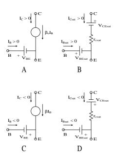
(A) Simple dc biasing model for an *npn* BJT in its forward linear operating region (see text for examples). (B) dc biasing model for an *npn* BJT in forward saturation. (C) Simple dc biasing model for a *pnp* BJT in its forward linear operating region. (D) dc biasing model for a *pnp* BJT in forward saturation.
