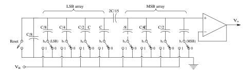
**FIGURE 10.6** A charge-scaling switched-capacitor DAC.
