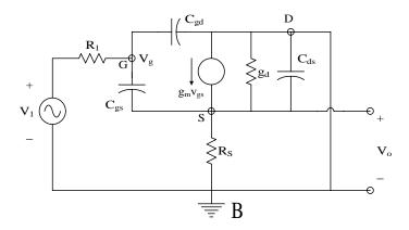
**FIGURE 2.50**(A) A JFET source-follower amplifier. (B) The HFSSM for the amplifier.
