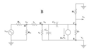
**FIGURE 3.7** (A) High-frequency SSM for the left-half BJT DA given common-mode excitation. (B) High-frequency SSM for the left-half BJT DA given difference-mode excitation.
