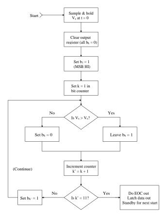
**FIGURE 10.13**Logical flowchart illustrating the steps in one conversion cycle of a successive-approximation ADC.
