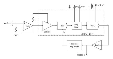
**FIGURE 12.14** Detailed block diagram of Du's PLL.
