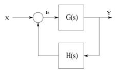
**FIGURE 5.5** A simple two-block SISO feedback system.
