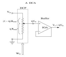
FIGURE 7.15 Schematic of a digitally controlled attenuator (DCA).
