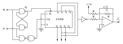
**FIGURE 12.12** A shift register-based digital phase-frequency detector.
