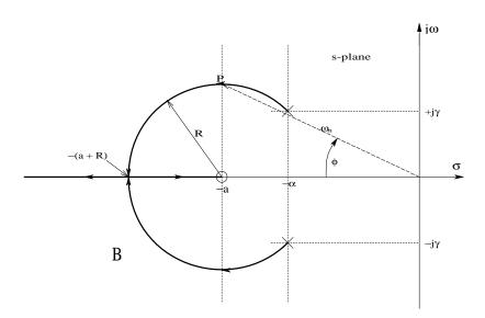
(A) The well-known circle root locus for a NFB system with two real poles an a high-frequency real zero. See text for discussion. (B) Interrupted circle root locus for the same NFB system with complex-conjugate poles at  $\mathbf{s} = -\alpha \pm j\gamma$ .
