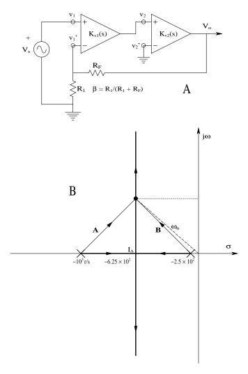
(A) Two op amps connected as a noninverting amplifier with overall NVFB. (B) Root-locus diagram for the amplifier. Note that unless a sharply tuned closed-loop frequency response is desired, the feedback gain,  $\beta$ , must be very small to realize a closed-loop system with a damping factor of 0.7071.
