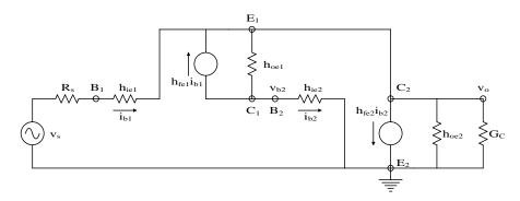
Top: feedback pair amplifier with load resistor,  $R_C$ , attached to common  $Q_1$  emitter +  $Q_2$  collector. Bottom: MFSSM of the feedback pair amplifier above. Analysis in text shows this circuit behaves like a super emitter follower.
