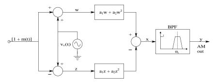
**FIGURE 11.5** Block diagram of a quarter-square multiplier used for amplitude modulation.
