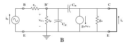
(A) The hybrid pi, high-frequency SSM for a BJT. A common-emitter configuration is assumed. (B) A hy-pi HFSSM circuit used to calculate a BJT's complex short-circuit output current gain,  $h_{f_i}(j\mathbf{w})$ , and  $f_{T_i}$  where  $\left|h_{f_i}(j2pf_T)\right| = 1$ .
