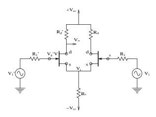
**FIGURE 3.2** A JFET differential amplifier. The circuit must be symmetrical to operate well.
