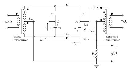
**FIGURE 12.4** The diode bridge PSR when diodes *c* and *d* are conducting, and *a* and *b* are blocking current flow.
