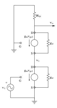
**FIGURE 2.38** MFSSM for the two-JFET cascode amplifier. See text for analysis.
