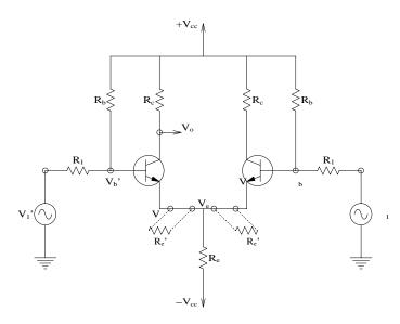
**FIGURE 3.6** A BJT DA. Note symmetry. The resistors  $R_{\epsilon}'$  are used to raise the DM input resistance.
