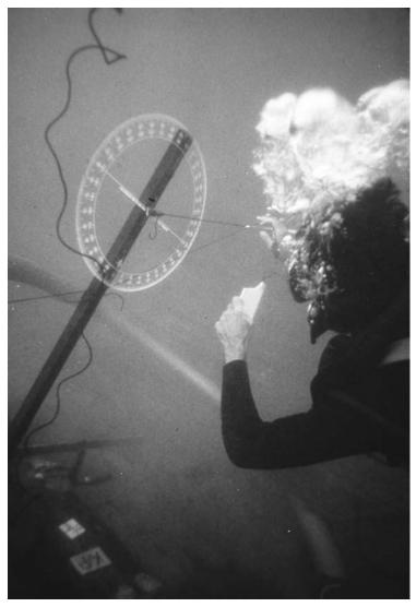
**Figure 4.1** Distance-angle measuring system. Circular protractor mounted on the keelson of the *Santo Antonio de Tanna*, a Portuguese wreck in Mombasa, Kenya. The protractor and tape measure were used to plot the curvature of the hull.
