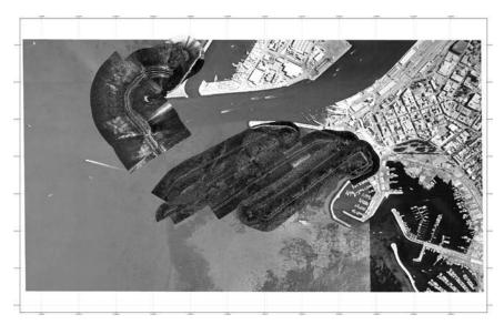
**Figure 7.6** Side scan sonar GeoTIFFs overlaying a georeferenced aerial photograph of Bathers Bay, Fremantle.
