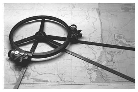
Figure 3.12 Station pointer used to resection sextant angles.
