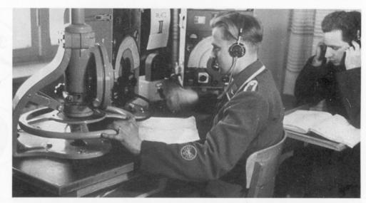
**Above:** An NCO Direction Finding operator operating radio direction finding apparatus.
