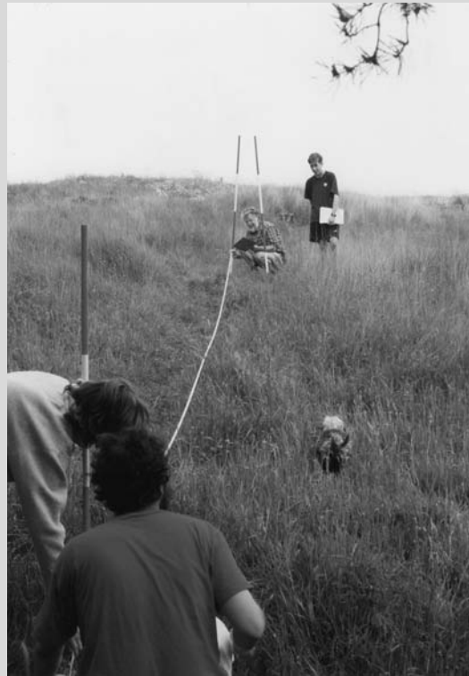
Figure 13.5 Students using tapes, ranging rods and clinometers to measure Painswick Beacon Hill Fort in order to construct profiles of the earthworks
