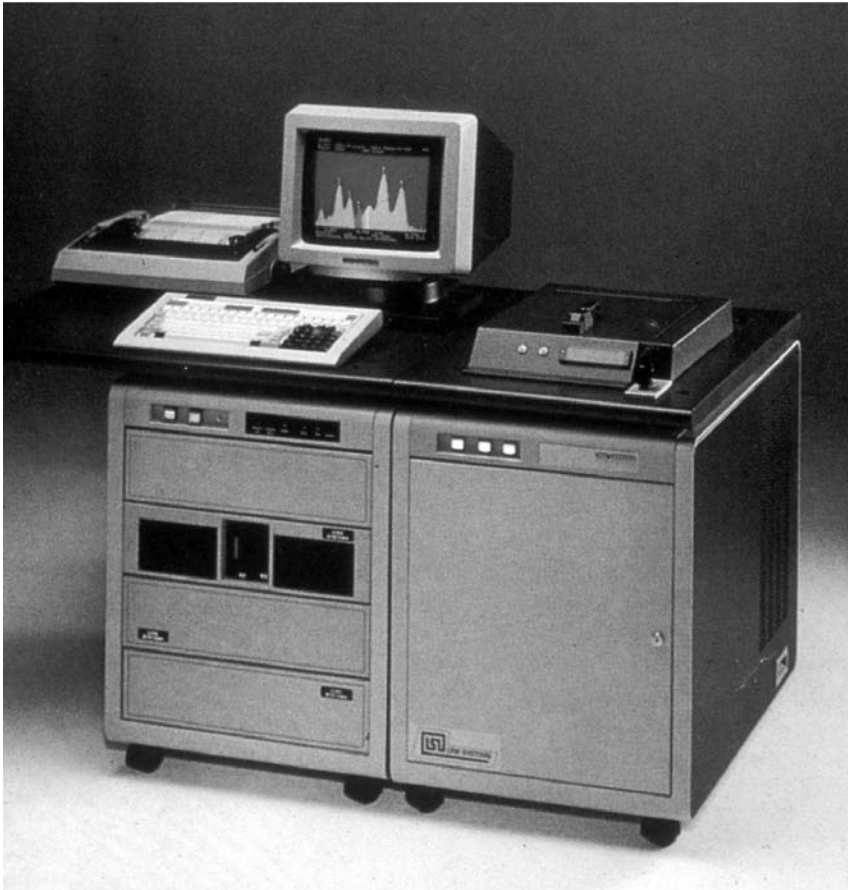
Figure 4.7 Link Systems XR200 energy-dispersive X-ray fluorescence (EDXRF) system. (Photograph courtesy of Jennifer Jones and Phil Clogg)
