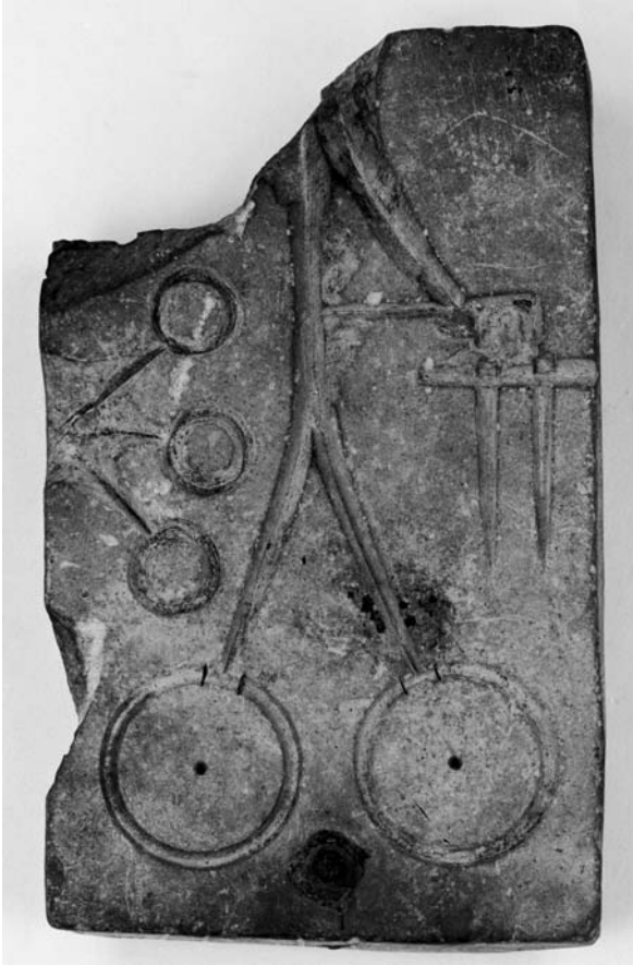
Fig. 6.6. Stone mould from Perth for casting the frames and pins of ring-brooches and other small rings. It was used with a 'partner'; one of the lead plugs that ensured a tight fit by matching a hole in the other half can be seen at the bottom. Broken off at the top is the in-gate into which liquid metal was poured to flow down the runners—when the metal had cooled and solidified the stones were separated, the rings and pins removed and filed smooth, and the surplus metal in the runners could be put back into the melting-pot for reuse. (Photograph reproduced by courtesy of Perth Museum & Art Gallery, Perth & Kinross Council, Scotland. Actual size.)
