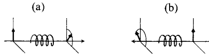
FIG. 3.23. Rotation of the plane of polarization of light traveling through a helix for two opposite directions of propagation.
