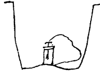
FIG. 3.4. One of Faraday's experiments with an electrified copper boiler ( FD 2: 408 ). The gold-leaf electrometer at the bottom of the boiler shows no sign of electricity.
