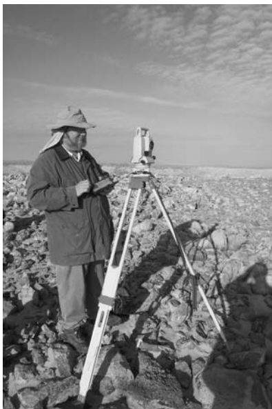
FIGURE 2.12 The use of total stations has revolutionized archaeological recording for both accuracy and speed. On the left, a crew member uses a small computer to coordinate information received from the total station. On the right, another crew member holds the prism pole at the point being recorded by the total station.
