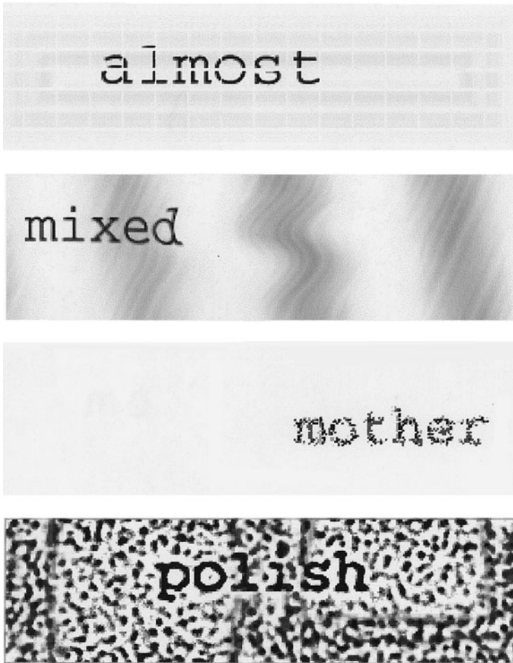
Fig. 7.1 CAPTCHA (Completely Automated Public Turing-Test to Tell Computers and Humans Apart). CAPTCHA aims to unmask web-bots posing as humans by asking them to recognize words and shapes against a backdrop of noise. Illustration by Christine Clark.
