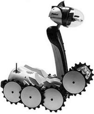
Fig. 4.2 Multipurpose domestic robot designed by Rodney Brooks and iRobot Corps. Described as a “remote presence” robot, the iRobot-LE can climb stairs and traverse most household terrain. The user controls the robot over the web, telling it where to go in the distant house. The top-mounted camera and microphone then send sound and vision back to the user, wherever she is in the world. Photo courtesy of Professor Rodney Brooks.
