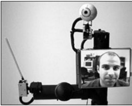
Fig. 4.5 A ProP (Personal Roving Presence device), designed by John Canny and Eric Paulos. The device acts as your representative at a distant site and provides gaze control, body control, posture, and dialogue. Photo courtesy of Eric Paulos.
