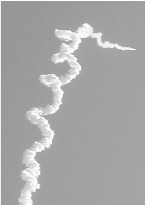
Fig. 1.8. Launch of the Japanese-American satellite Astro-E. The corkscrew-shaped exhaust trail is a certain sign of trouble. (Image used by permission of Dr. Damian Audley.)
