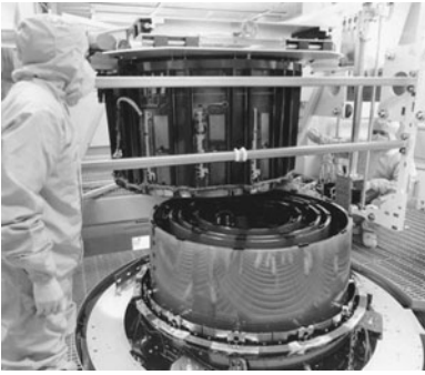
Fig. 3.5. Assembly of the polished mirrors. The arclike appearance of the assembled mirrors is captured in the artist's impression of Fig. 1.3 in chapter 1. (Courtesy Kodak Corporation.)
