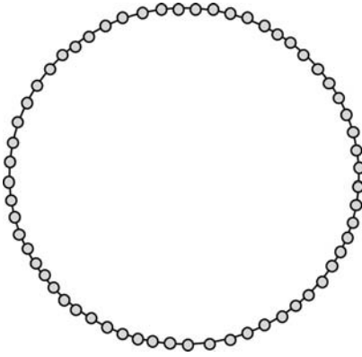
FIGURE 15.4. An example of a regular network. This network is a ring of nodes in which each node has a link to its two nearest neighbors.
