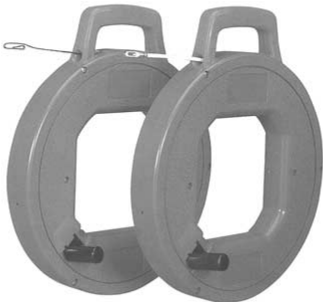
FIGURE 11.12 Fish tapes housed in spools.
