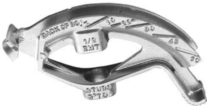
FIGURE 11.8 Detail of conduit bender head.
