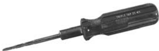
FIGURE 11.7 Triple-tap tool taps three hole sizes, and cleans and chases burred threads.
