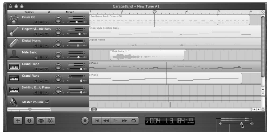
Figure 4-10: Adjusting the master volume for the song (which is too loud, as shown by the volume level meter).
