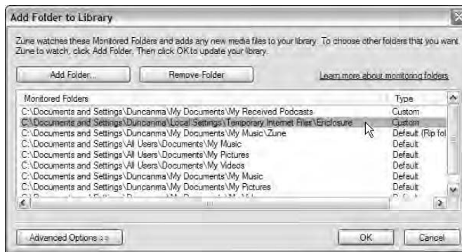
Figure 10-22: Add the Enclosure folder to your Zune library to pick up any podcasts in that folder.
