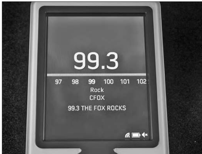
Figure 4-19: Your Zune receives extra info, in addition to the normal FM audio.
