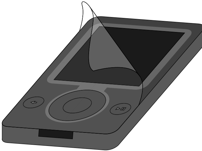
Figure 19-3: Screen protectors are a plastic film that sticks to the entire top surface of your Zune and helps you avoid scratches.
