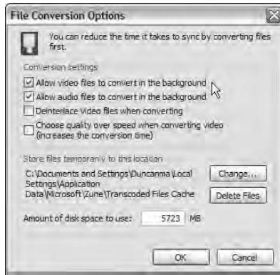
Figure 12-10: The File Conversion Options dialog box lets you control background audio and video encoding.
